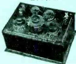
An efficient but inexpensive set employing a detector valve with reaction and a stage of L.F. amplification. It will give good loud-speaker results up to about 20-30 miles from a B.B.C. main station or approximately 100 miles from Daventry.
