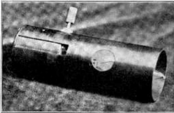
FIG. 11.—CELL FOR TRANSFORMING LIGHT FLUCTUATIONS INTO ELECTRIC CURRENTS
