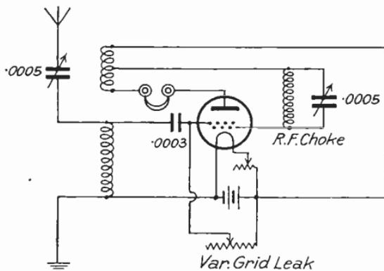
FIG. 1.—THE UNIDYNE CIRCUIT FOR H.T.—LESS RECEPTION
