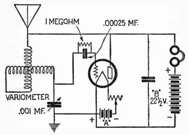
Fig. 21. An ultra andion circuit illustrating aspecitive feedback.
