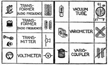
The left shows a picture of the apparatus while the right shows the symbol used in all radio hook-ups.
