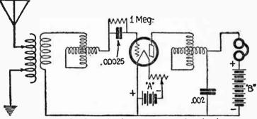
Fig. 22. The three circuit tuner regenerative circuit.
