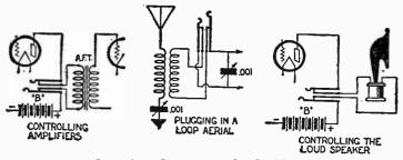
Fig. 34. Several applications of the double circuit jack.
