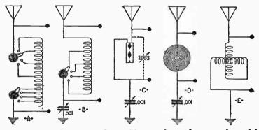
Fig. 9. How inductances and capacities may be used to tune the aerial circuit.
