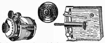
Fig. 13. Variable condensers of the three styles as mentioned. Left to right they are, the intersecting plate with vernier device, the mica dielectric, and the book type.
