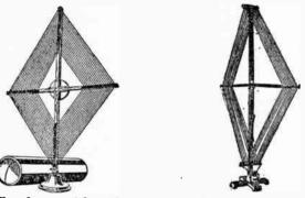
Fig. 7. Two loop aerials. The one on the left is known as the spiral type and the one on the right, the Solenoid type.
