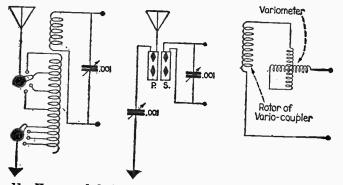
Fig. 11. How coupled circuits are connected and tuned. The first is a tapped vario-coupler, the second honeycomb coils, and a third a variometer.
