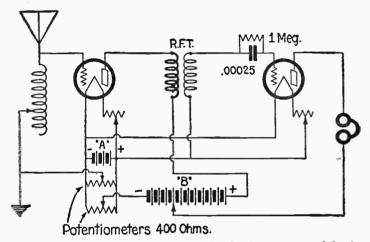
Fig. 24. A circuit employing one stage of radio frequency amplification and a detector tube.
