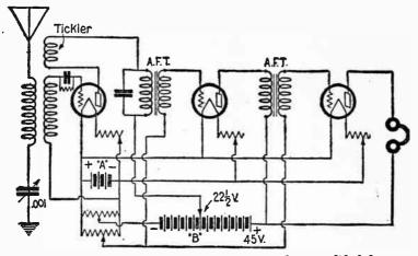
Fig. 31. Diagram of a regenerative circuit further amplified by two stages of audio frequency amplification.
