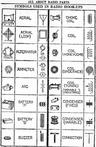
The left shows a picture of the apparatus while the right shows the symbol used in all radio hook-ups.
