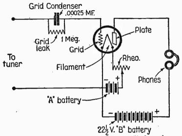
Fig. 17. Circuit showing how the vacuum tube is utilized as a detector
