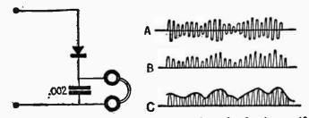
Fig. 15. Connections of a crystal detector and graphs showing rectification of radio frequency currents and the resultant audio frequency current that actuates the phones.
