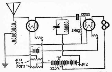
Fig. 29. Tuned impedance coupling for radio frequency amplification.
