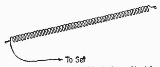
Fig. 6. The spring antenna is installed by simply stretching it between two opposite corners of a room and bringing a lead down to the set.
