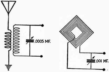
Fig. 12. The untuned primary circuit and method for tuning a loop aerial.
