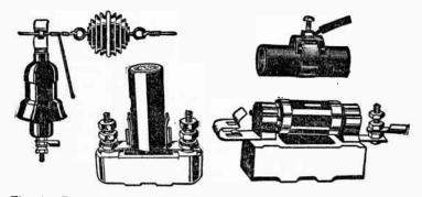
Fig. 4. Different types of vacuum lightning arresters and a ground clamp. The arrester on the left is especially designed to be used out of doors and therefore it is attached directly to the antenna wire as shown.
