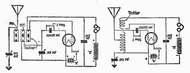
Fig. 20. Amplification by regeneration. The circuit on the left is known as the "Honeycomb coil tickler feedback" and the one on the right the "Single circuit with tickler feedback."
