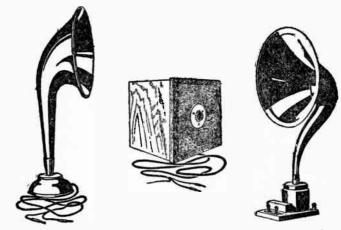
Fig. 36. Popular types of loud speakers. They are, in orden, the receiver unit, adjustable, and power talkers.
