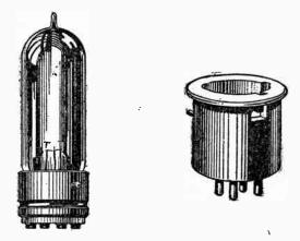
Fig. 19. The U. V. 199 vacuum tube and adapter to fit the standard socket.
