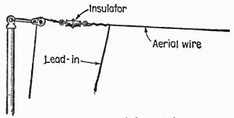
Fig. 2. How an insulator is attached to a single wire antenna.
