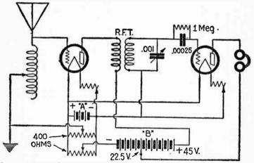
Fig. 28. A tuned secondary circuit of a transformer as applied to radio frequency amplification.
