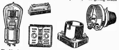
Fig. 16. A vacuum tube and component parts which are used in conjunction with it as a detector. A grid leak, condenser, socket, and a rheostat are shown to the right of the tube.
