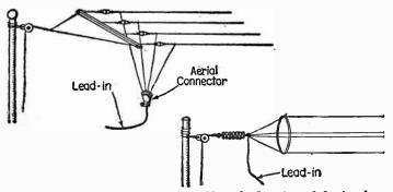
Fig. 3. Insulating multi-wire aerials. Note the location of the insulators and the place where the lead-in is taken off from in each case.
