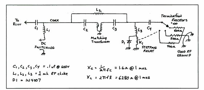
Figure 3. Basic DC switching and isolation techniques
