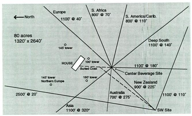
Figure 1. Beverage layout at VE6JY
