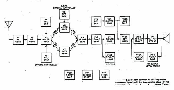
Figure 3: SP-600-JX-17 Block Diagram
