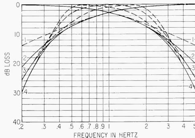
Only by applying feedback over the dividing network, or otherwise inducing interaction, can the true response form be achieved. When it is, the amplitude and phase relationship will follow the minimum-phase network laws, and thus behave just like the prototype electrical crossovers.
