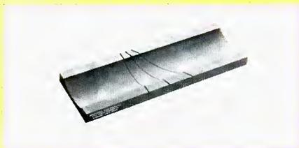
● This editing block is designed to handle two-inch tape and provide either straight or angular cuts. It holds the tape securely, yet is as simple to use as conventional ¼-inch tape blocks. It is hard anodized aluminum with a satin finish. Length is 7¾ inches and the height is ½ inch. Delivery is immediate.
