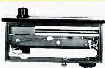
● A low-impedance straight-line ladder attenuator offers a smooth mechanical slide system. A set screw adjusts the exact tension to give a light feel. The resistive elements and related wiper mechanics are designed to eliminate contact bounce and to increase contact pressure to allow wiping through the usual atmospheric coating without making the movement stiff. The Gliss 7011 is available as a retrofit for most existing straight-line mixers.
