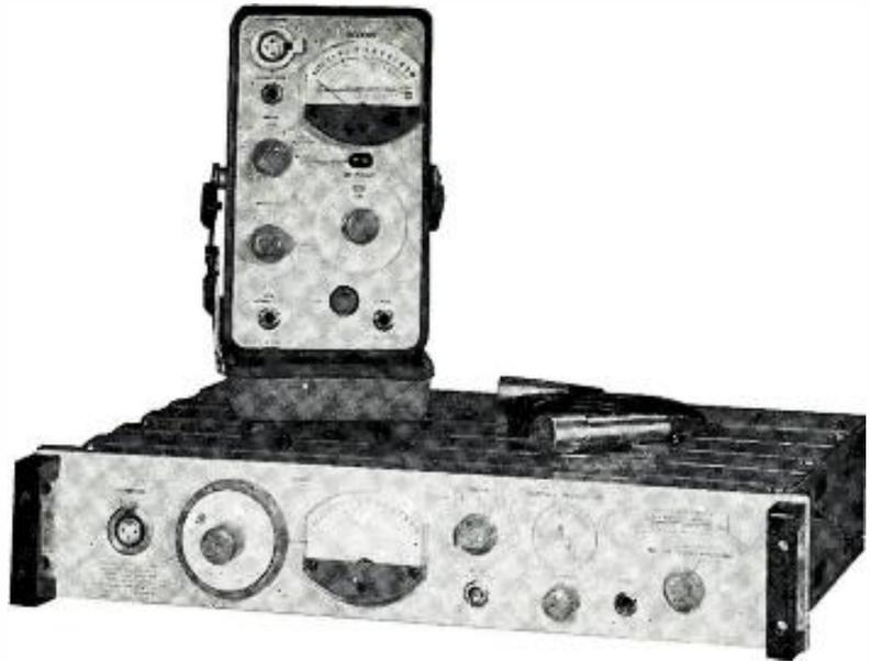
● Specifications defined by the International Electrotechnical Commission in IEC 179, 1965 are met by the new type 1561 precision sound-level meter. A new ceramic microphone is used, the instrument is all solid-state, provides flat response from 20 Hz to 20 kHz for measurement of sound-pressure level, and has a jack that permits connection
