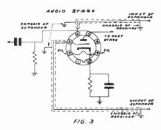
the expander. It may be convenient to place a phone jack in the expander chassis for plugging in the pick-up unit. If a short circuiting jack is used and the switch on the jack connected in such a way that the expander input is disconnected from the receiver, when the phone plug from the pick-up is placed in the phone jack, the necessity of a separate switch is eliminated.
