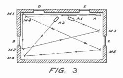
a way that it will fall upon a photoelectric cell, it will actuate the cell. By the use of mirrors (Fig. 3) the arc of a room can be covered so thoroughly that no one can enter without intercepting the beam of ultra violet light. When this beam is intercepted, some type of burglar alarm is set off. The use of this type burglar alarm has become very popular.
