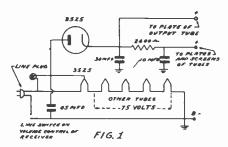
The circuit of Fig. 1 is typical of receivers using a 3525 or similar tube as a rectifier. The filaments are connected in series. The pilot light is connected across part of the 3525 filament. The 3525 is a special tube made so that the pilot light can be connected as indicated. The size of this light, however, is important and the value specified should be used when it is replaced.
