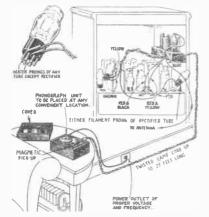
FIG. 2. Diagram showing how the RCA phonograph oscillator and a record player employing a high-impedance magnetic pick-up are connected to a typical A.C. radio receiver.
