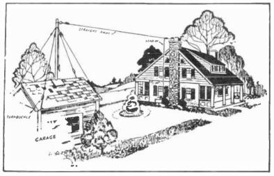
Fig. 1. A simple, effective Antenna System
