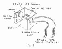
Recall that I said that there were three ways to connect a tone control. Personally I would not use the grid to chassis connection, as the long leads from the grid may affect the action of the audio amplifier system. Use either the plate to chassis or plate to plate connection.
