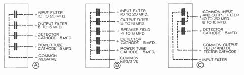
FIG. 5. Typical condenser block diagrams for universal receivers.
