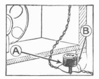
Connect these two cut ends to the terminals of an AMPERITE adapter socket as shown by lines "A & B" or to any standard UX tube socket. If a tube socket is used, make connections to either two opposite terminals, leaving the remaining two terminals blank.
