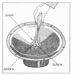
FIG. 3. Re-centering a loudspeaker voice coil with the aid of celluloid shims.
