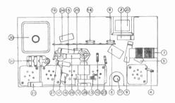
This particular type of pictorial inyout diagram, showing locations of parts on the chassls but omitting all wiring, is typical of those found in the service manuals for some Philco receivers.
