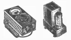
Unit for reducing 32-volt output of farm power plant to 6 or 2 volts for tube filaments of a battery receiver. This self - rectifying vibrator unit boosts 2, 6, 12 or 32 volts D.C. to higher D.C. values for farm radios.
