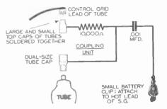
FIG. 1. Standard coupling unit, used for making a signal generator connection to a control grid lead of an R.F. tube (in modern R.F. tubes the control grid invariably goes to a top cap). The grounded S.G. lead goes to the receiver chassis; the other S.G. lead, commonly called the hot lead, goes to the battery clip on this coupling unit.
