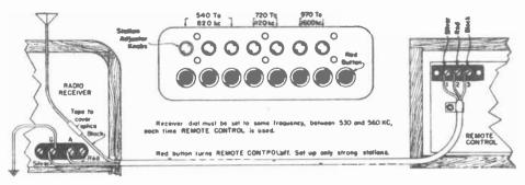
FIG. 2. Connections for Melasner remote control tuner.
