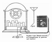
FIG. 1. How to Connect Signal Generator.
