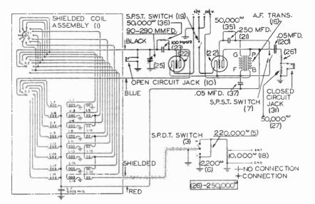
FIG. 5. Circuit diagram for signal generator. Note colors of RCA coil assembly leads.
