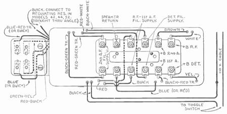
Fig. 3-View of Power Unit used in AK Models 40, 42, 44 and 52, showing connections from sealed container to panci assembly, rectifier socket and regulating resistance.
