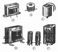
FIG. 2. Defects in colls and transformers like these are common causes of receiver failure. Airon-core coll, also called a choke coll or filter choke; B-simple coll wound on wood core; Csame coll as at B, in metal housing; D--tron-core transformer; E-transformer made up of several colls wound on bakelite tubing; F--transformer in metal housing.
