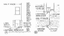
FIG. 7. Lead-in and ground connections.
