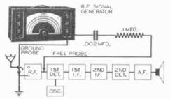
FIG. 1. Block diagram of a superheterodyne receiver, showing a signal generator connection to the first detector for locating a defective stage.
