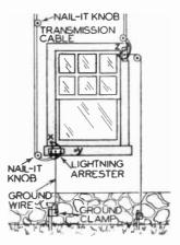
FIG. 2. This sketch illustrates various methods of bringing the transmission cable through the window or window frame into the house. Either screw insulators or nail-it knobs can be used to support the transmission cable along the sides of the house.
