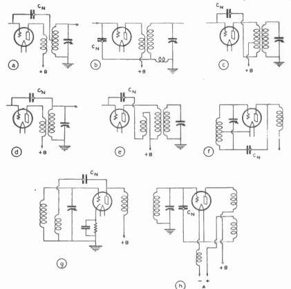
Fig. 1. Common methods of neutralizing feed back; all have the same adjustments.
