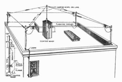
FIG. 6. Installation involving 4 master antenna systems on the roof of a large apartment building. Each system serves one vertical row of 20 apartments.
