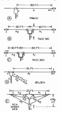
FIG. 1. The essential features of five basic types of all-wave, noise-reducing antennas are shown here in simplified form. In each case the exposed aerial wires which serve to pick up the radio signals are designated by the letter A; antenna transformers are designated as T; insulators are designated as I; transmission cables are designated as C. The heavy arrows indicate the directions from which radio signals are received best in each case.
