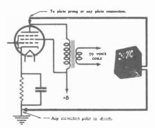
F10. 2. How to Connect the Output Indicator to a Single Tube Output Stage.
