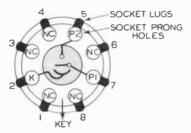
FIG. 7. Socket connections for type OA4-G tube as viewed from the bottom of the standard octal socket.
