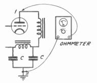
FIG. 3E. If you test continuity in this case, and C happens to be an electrolytic condenser, the ohmmeter needle may creep up or down scale. Electrolytic condensers have polarity. Always connect the ohmmeter so the needle creeps up scale.
