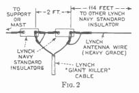
Always follow the instructions sent with a kit, for manufacturers make improvements or suggestions that are important if you want the best results. The instructions with this kit indicate that the straight-away antenna must be cut to be exactly 114 feet long. Furthermore, the transmission line or cable is connected to one end of the antenna straight-away. This will mean that this support should preferably be directly above the lead-in window.
