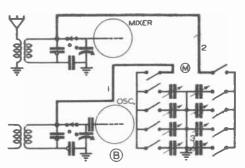
FIG. 6. Fuli-automatic (A) and semi-automatic (B) connections of a trimmer-type push-buttom tuner to an all-wave superheterodyne having a two-section variable tuning condenser.
