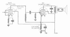
FIG. 3. Detector and output stage of a universal receiver, showing a simple but entirely satisfactory method for getting a low positive acreen grid voltage for the detector tube.
