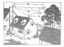
Tynical installation of an RCA Spider Web Antenna System.
