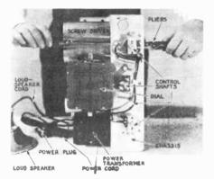
FIG. 7. Learn to handle a chassis in this manner when tightening loose bolts.
