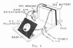
as shown in Fig. 4. This set-up is easier to use because of its compact assembly. You need the 0-5 milliammeter, the 10,000 ohm potentiometer, the two probes, two Fahnstock clips, and a  $22\frac{1}{2}$  volt battery. I suggest that you buy a small C battery. Connect these parts in series as shown.
