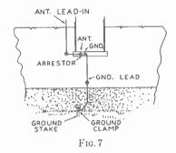
nected to the ground terminal of the lightning arrester. The other end is extended out along the bottom of the ditch. After you have completed the ditch, then the 50 foot length of wire may be laid in and the original earth used to cover the wire.
