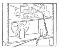
Mount the adapter or socket at any convenient place inside the cabinet. Insert the proper AMPERITE Line Voltage Control tube and the receiver is ready for operation. When making the above connections, first disconnect the house line plug.
