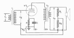
FIG. I. Basic inverse feedback circuit.
