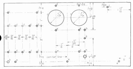
FIG. 4. Layout for 97s" x 47s" subpanel (bottom view). See tables for hole diameters.
