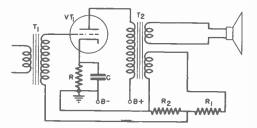
FIG. 4. Circuit using extra winding for feedback.
