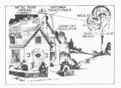
FIG. 1. All-wave antenna installation employing s chimney and a tree as supports.
