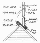
FIG. 5. Suggested construction for a wood mast which is to be at the peak of a roof.
