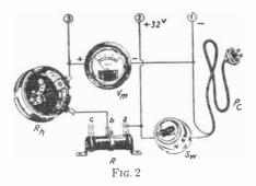
should be a 100 ohm, 25 watt resistor,  $R_h$  should be a 25 ohm,  $\frac{1}{2}$  ampere resistor. Observe that R is a movable tap or semi-fixed resistor, while  $R_h$  is a power rheostat.
