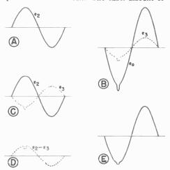
FIG. 2. Curves showing result of inverse feedback.
