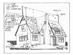
FIG. 2. All-wave antenna installation employing two self-supporting iron masts on a house roof.
