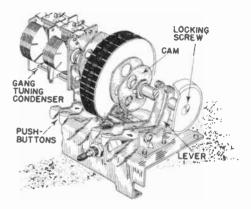
FIG. 5. Typical cam-and-lever mechaniam used in mechanical automatic tuning systems.
