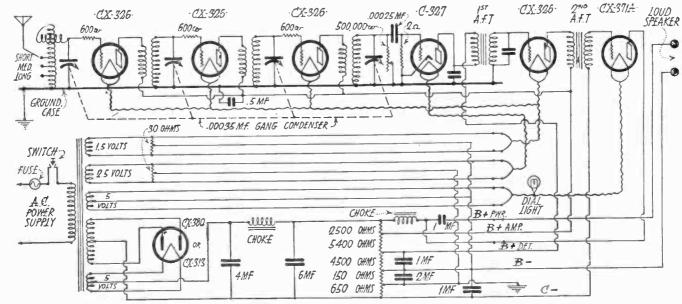
Fig. 3-A Typical AC Receiver.
