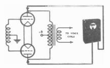
FIG. 4. How to Connect an Output Indicator to Sets Having Push-Push or Push-Pull Output Stages.
