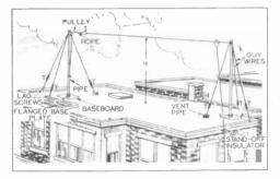
FIG. 3. All-wave antenna installation employing guyed iron pipe masts located on the flat roof of an apartment building. Insulators are designated as I, and turn-buckles as T.
