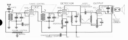
FIG. 1. Signal circuits of a typical universal T.R.F. receiver. Alignment simply involves tuning in in station, then adjusting trimmer condensers CI and C2 (mounted on the gang tuning condenser) for maximum output volume.
