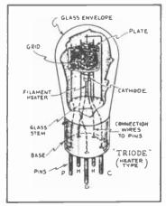
Fig. 2. An exploded view of a heater type tube
