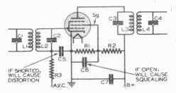
FIG. 2. Typical I.F. amplifier stage.
