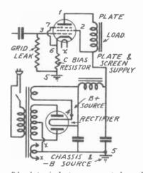
FIG. 3A. A typical stage connected to the main supply. Continuity tests should be made between 1 and 4, 2 and 4, 3 and 5, . 6 and 5, 7 and 5.
