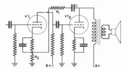
FIG. 7. Plate to cathode feedback over two stages.
