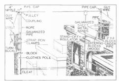
FIG. 4. All-wave antenna installation in which an extension mast on a clothes pole in the backyard serves as one support.
