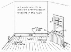
FIG. 7. Example of receiver location which requires extension of power, antenna and ground leads.
