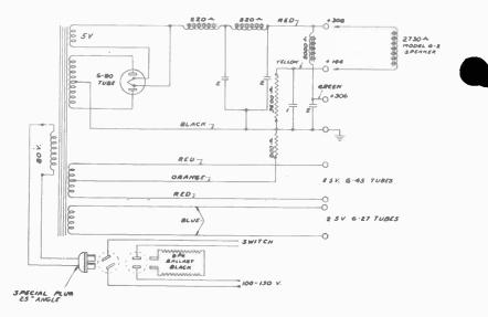
SCHEMATIC DIAGRAM OF SPG POWER UNIT
