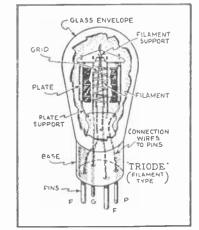
Fig. 1. An exploded view of a filament type tube
