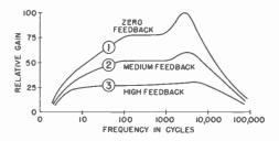
FIG. 3. How inverse feedback improves response.
