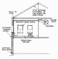
FIG. 2. When a standard outdoor antenna cannot be installed for any reason, consider one of the makeshift antennas illustrated here.
