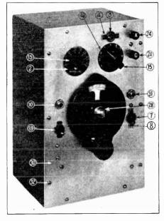
FIG. 1. The completed signal generator, designed and built in the N. R. I. Labora-tory, fits into 7" x 1034" x 532" cabinet.
