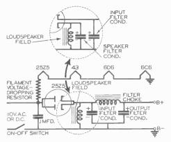
FIG. 2. One type of power supply circuit commonly found in universal receivers. Alternative loudspeaker field coil connections are shown inside the dotted circles.
