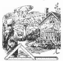
How the pitch of a roof can be closely estimated from the ground by using a folding ruler. Courtesy of Popular Mechanics
