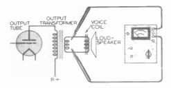
FIG. 2. Output indicator connections to the voice coil of a dynamic loudspeaker. A multimeter is here being used as an output indicator.
