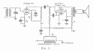
fective. The plate and screen voltage of the detector tube is measured in the same way as on the power tube except that the —probe is placed on the cathode of the tube. If there is no cathode to screen or plate voltage place the —probe on the chassis. If voltages are then available,
