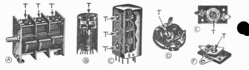
FIG. 9. Screw heads and hexagonal nuts like those marked T in this illustration are for alignment or sume-up purposes, and must not be souched while overhauling a chassis. You will find these alignment acrews on gang tuning condensers as at A, on top of a metal coil shield as at B, at the side of a coil shield as at C, and on separate parts like those at D, B, and F, which are mounted directly on the chassis.
