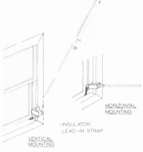
FIG. 6. Tobe window pole antenna, made by the Tobe ibeutschmann Corp. for use in apartment buildings; it is especially useful to radio dealers who need a temporary antenna for a demonstration or for use with a rental receiver. The clamp attaches to the window frame, and permits mounting the 8-foot antenna rod in either a horizontal or a nearly vertical position.
