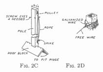
base to fit flat or sloping roofs. Figure 2B shows a three piece one-inch pipe mast fitting consisting of pulley, collar for guy wircs and adjustable base. For those who prefer to make their own mast, as shown in Fig. 2C, you will need:
