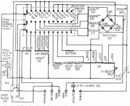
FIG. 8. Follow this Circuit Diagram Closely when Wiring Your Multimeter.
