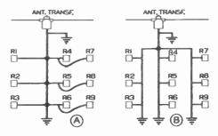
FIG. 3. Two methods for connecting receivers to a master all-wave antenna.
