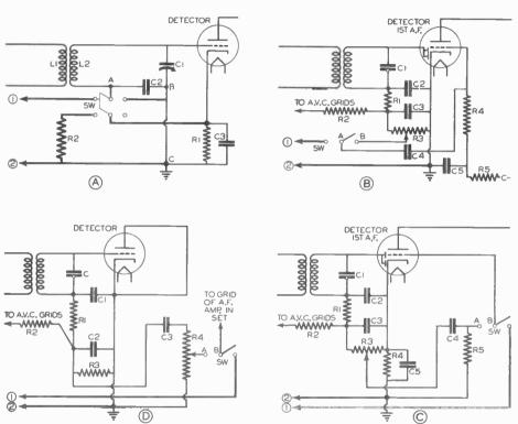
FIG. 5. Four typical detector circuits; changes required to make a direct pick-up connection are indicated in heavy lines. The leads from the pick-up device should go to points 1 and 2.
