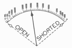
FIG. 1. Typical ohmmeter scale, with the pointer indicating a reading of 30,000 ohms. Normal or no-current position of pointer is at extreme left, as indicated by the dotted line. Maximum-current position of pointer is at extreme right, corresponding to zero resistance or a shorted part. Note that an ohmmeter scale has its lowest value at the *right*, whereas voltmeters and ammeters ordinarily have the lowest value at the left.
