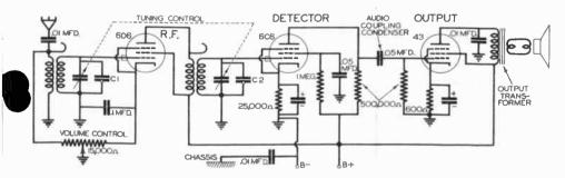
FIG. 1. Signal circuits of a typical universal T.R.F. receiver. Alignment simply involves tuning in in station, then adjusting trimmer condensers *Cl* and *C2* (mounted on the gang tuning condenser) for maximum output volume.
