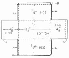
F1G. 3. Layout of copper shielding screen. Cut on heavy lines. Flaps A and B are %s" wide. Bend flaps A up on dotted lines; bend sides and ends up, then place in cabinet and bend flaps B down over the top edges of the S.G. cabinet.
