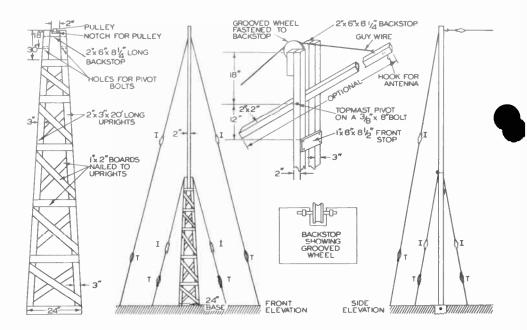
FIG. 5. Suggested design for a thirty-foot high wooden mast. Insulators are designated as I, and turn-buckles as T.
