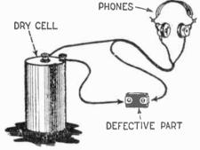
Fig. 2—Head-phones and Dry Cell Method of Testing Defective Apparatus.
