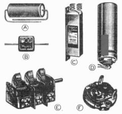
FIG. 3. Examples of condensers which may cause receiver failure. A--tubular paper condenser; B--mica condenser; C and D--electrolytic condensers; E--three-section variable tuning condenser; F--trimmer or semi-adjustable condenser.
