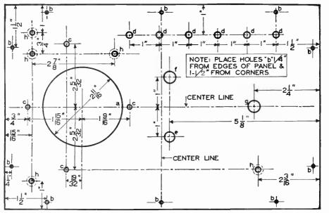
Fig. 2. Layout of the Front Panel of the Multimeter.
