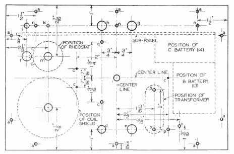
Layout for 10-13/16" x 7-1/16" aluminum front panel (front view). Refer to F1G. 2. dotted lines when mounting parts on the panel. Locate holes "a" 5/16" from outside edges and  $1\frac{1}{2}$ " from nearest corner.
