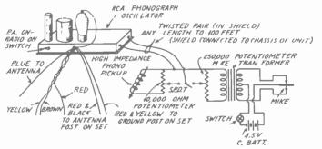
FIG. 4.—The yellow and brown leads are connected to the heater prongs of any tube except the rectifier by means of tube prong clips; the red lead is connected to either one of the filament prongs of the rectifier tube.
