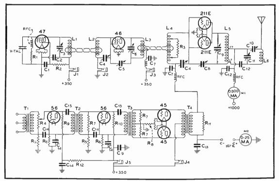
FIG. 12. The 50 Watt Phone Transmitter.
