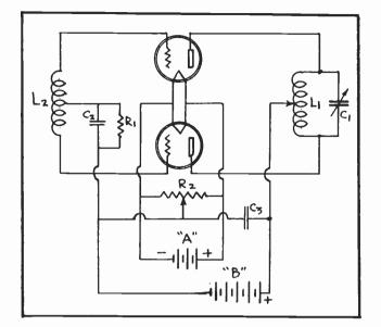
FIG. 11 The Push-Pull Oscillator.
