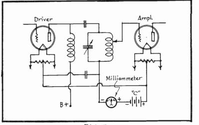
FIG.3 Milliammeter Connection When Using Tuned-Grid Circuit.
