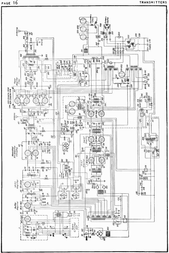
FIG. 8 R.C.A. Victor 1-Kw. Broadcast Transmitter.
