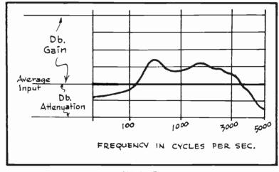
FIG. 5. A Frequency Response Curve
