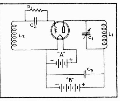
FIG. 9 T.N.T." Circuit. The
