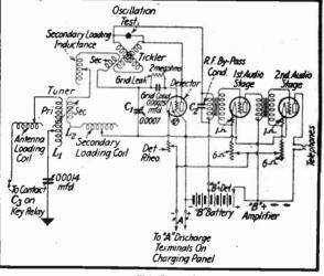
FIG. 14 The Receiver Diagram.
