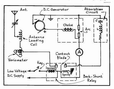
FIG. 14 The Arc Transmitter.
