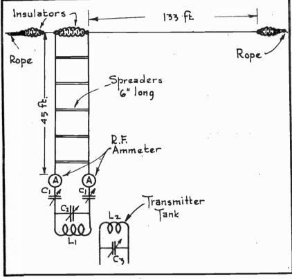
CURRENT LOOP WILL ALSO OCCUR AT THEIR INPUT ENDS BO THAT THE PHASE RELATION THROUGH-OUT THE SYSTEM MAY FOR BE CORRECT. THIS REASON, EACH WIRE OF THE FEED-ER 18 MADE ONE-HALF WAVELENGTH LONG. THIS AL80 PERMITS SERIES TUNING, WHEREAS IF THE FEEDERS SHOULD ONLY BEONE-QUART-ER WAVELENGTH LONG IT WOULD BE NEO-ESSARY TO INSTALL A PHASE - REVERBER IN THE FORM OF A TUNING PARALLEL CIRCUIT AT THEIR INPUT END.
