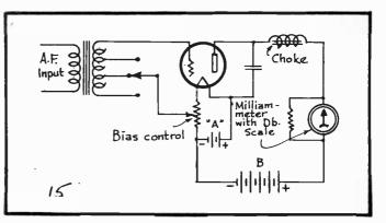
FIG. 15 Application of the V.T. Voltmeter as a Volume Indicator.
