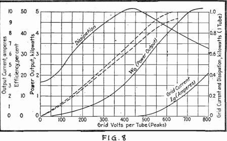
Dynamic Characteristic Curves of Two W.E. 279 A Tubes Operating in Push-Pull.
