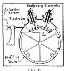
Synchronous Rotary Discharger.
