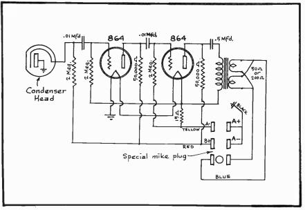
FIG.8 The Microphone Head Amplifier.
