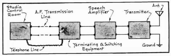
FIG. I Arrangement of Broadcast Transmitter Equipment.
