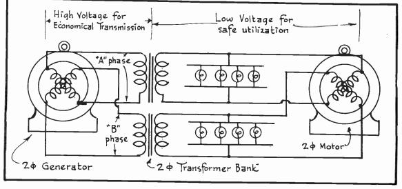
FIG. 4 A Two-Phase, Four-Wire System.
