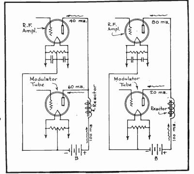
FIG. 7 Diagrammatic Explanation of the "Constant Current" Principle.
