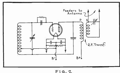
JUST AS ANY CHANGE IN THE DIELEC-TRIC SPACING BETWEEN THE PLATES OF A CON DENSER CAUSES A CHANGE IN CAPACITANCE, 80 ANY CHANGE IN SPACING BE-TWEEN THE TWO FEEDER WIRES DUE TO WIND, FOR EXAMPLE, WILL CAUSE A CHANGE IN CAPACITANCE WHICH WILL CHANGE THE RESONANT FREQUENCY OF THE SYSTEM. SINCE Α RESONANT CONDITION IN A SECONDARY COIL 18
