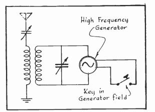
FIG.12 Transmitter Circuit With High-Frequency Generator.
