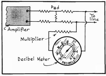
FIG 16 Application of the D.B. Meter.
