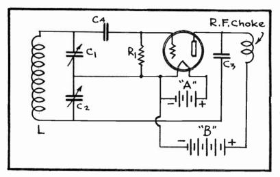
THE FEED-BACK E-FFECT IS INFLUENCED BY THE CAPACITY OF CONDEN-SERS  $C_1$  and  $C_2$  and the FRE QUENCY OF OSCILLATION IS DETERMINED BY THE INDUCTANCE VALUE OF COIL L IN CONJUNCTION WITH THE CAPACITIVE VALUES OF CONDENSERS  $C_1$  and  $C_2$ .
