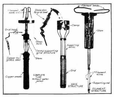
FIG. 9 A Water-Cooled Tube.
