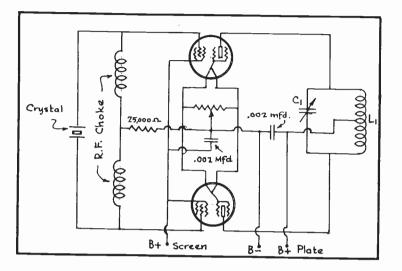
LOW GRID-PLATE CAPAC-ITY AND THEREFORE HAS A TENDENCY TO REDUCE THE FEED-BACK SOME-WHAT. IN ADDITION, PEN TODES ARE CAPABLE OF DELIVERING FAIRLY LARGE POWER OUTPUTS WITH A SMALL EXITING GRID VOLTAGE.
