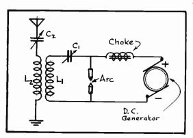
FIG.13 Simple Arc Transmitter. AS WELL AS ACROSS THE TUNED CIRCUIT, TO RISE UNTIL THE CONDENSER C 1 IS FULLY CHARGED.
