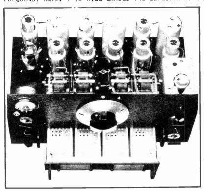
FIG.2 The National Receiver Removed from the Cabinet
