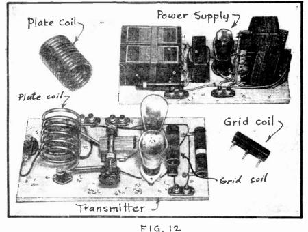
The Push-Pull Transmitter and Power Supply.
