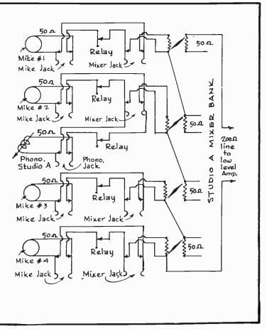
FIG. 9 The Typical Mixer Circuit.
