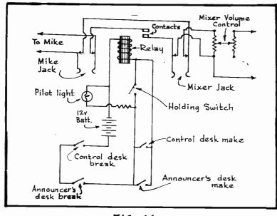
FIG. 14 Details of Microphone Control Circuit.
