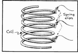
NSFORMER IS GENERALLY SPACE-WOUND WITH LARGE DIAMETER BARE COPPER WIRE OR ELSE COPPER TUBING BO THAT THE COIL BECOMES SELF-SUPPORTING AND REQUIRES NO WINDING FORM. SPRING CLIPS ARE THEN USED AS ILL-USTRATED IN FIG. 4 SO THAT THE COM NECTIONS TO THE COIL CAN BE VARIED IN A CONVENIENT MANNER BO THAT AS MANY TURNS OF THE COIL AS NECESSARY CAN BE INCLUDED IN THE TUNED CIR-CUIT IN ORDER TO OBTAIN THE DESIRED INDUCTANCE VALUE.
