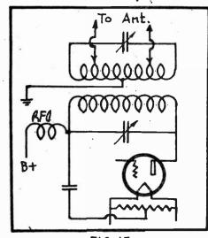
FIG. 15 Untuned line Coupled to Single-Tube Output. AT A TIME UNTIL THE TUBES ARE DRAWINGTHEIR NORMAL PLATE CURRENT.
