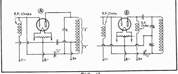
FIG. 12 Two Methods of Neutralizing.
