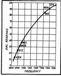
FIG.11 A Calibration Curve. DIAL - IF IT DOESN<sup>1</sup> T,TURNS CAN BE ADDED TO OR TAKEN OFF THIS COIL.
