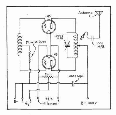
FIG. 13 Circuit of the Push-Pull Transmitter.
