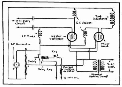
FIG. 10 Application of the Relay Key.
