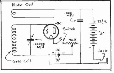
FIG. 9 Circuit Diagram of the Monitor.
