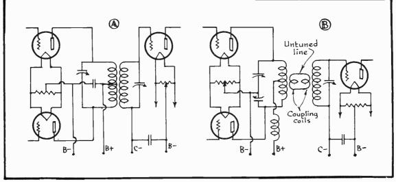
FIG. 11 Single Tubes Driven By Push-Pull Stages.
