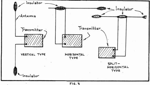
Three Fundamental Types of Hertz Antenna.
