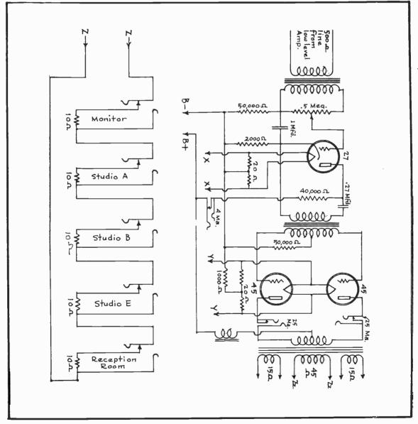
FIG. 13 The High-Level Amplifier.
