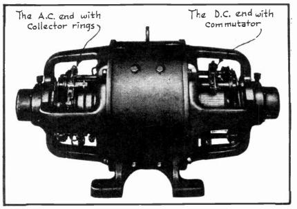
FIG. 26 A Synchronous Converter. Showing the A.C. and D.C. Ends.
