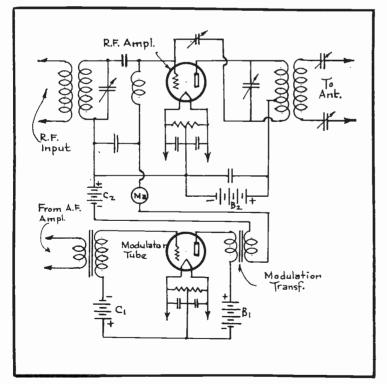
FIG. 10 Grid Modulation.
