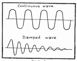
FIG.9 Continuous and damped waves.
