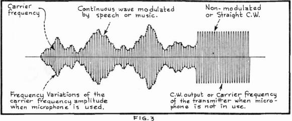
Modulating the Carrier Frequency.
