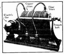
FIG.7 Quenched Spark Discharger.
