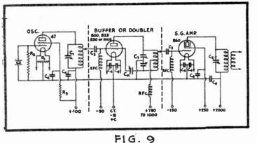
Application of Screen Grid Tube as Final Amplifier.
