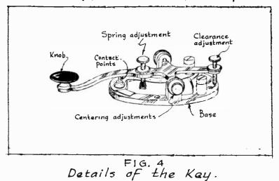
CLOSE THE CONTACT POINTS OR A CLEARANCE BETWEEN THE POINTS OF ABOUT 1/32" OR SLIGHTLY MORE. THE ADJUSTMENTS ASHERE GIVEN ARE ONLY AVERAGE AND CAN BE VARIED TO BEST SUIT THE INDIVID-UAL OPERATOR SO AS TO PERMIT HIM TO SEND THE CLEAREST SIGNALS POS9-IBLE.
