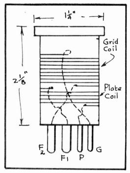
FIG. 10 The Monitor Coil.
