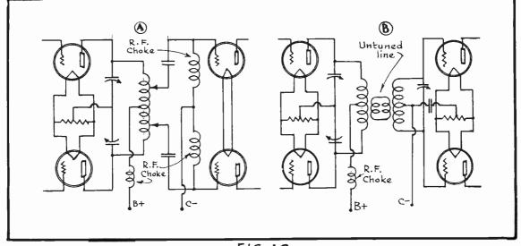
FIG. 10 Interstage Coupling Between Push-Pull Amplifier.
