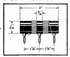
FIG. 14 Details of the Grid Coil.
