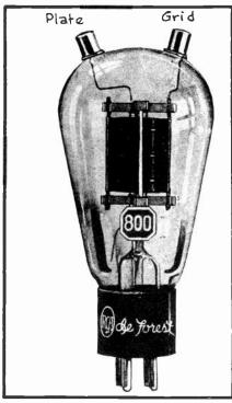
HIGH FREQUENCY CIRCUITS. THE MOST INTEREST-ING FEATURE OF THIS TUBE IS THAT THE GRID AND PLATE CONNECTIONS ARE MADE AT TWO METAL CAPS WHICH ARE PLACED ON THE CREST OF THE GLASS BULB. THIS FORM OF CONSTRUCTION RE-DUCES THE GRID-PLATE CAPACITY OF THE TUBE AND ITS CONNECTING CIRCUITS AND WHICH IS OFVITAL IMPORTANCE IN CIRCUITS OPERATING AT HIGH FRE-QUENCIES. AT THE SAME TIME, GOOD INSULATIVE PROPERTIES ARE ALSO INTRODUCED BY THIS ARR-ANGEMENT.
