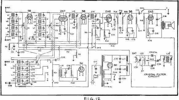
2.5 OR 6.3 VOLT SERIES. TWO STAGES OF TUNED RADIO FREQUENCY AMPLIFICATION ACT AS A PRE-SELECTOR AHEAD OF THE FIRST DETECTOR.
