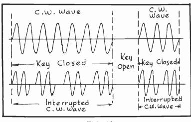
FIG. 11 The Interrupted C. W. Wave. INCOMING SIGNAL FREQUEN-CY TO PRODUCE THE INTER-MEDIATE FREQUENCY, ONLY THAT IN THE CASE OF THE RECEPTION OF C.W. CODE SIGNALS, THE BEAT FREQUEN CY IS IN THE AUDIBLE RANGE. THIS SUBJECTWILL BE EXPLAINED MORE THOR-OUGHLY IN A LATER LESSON.
