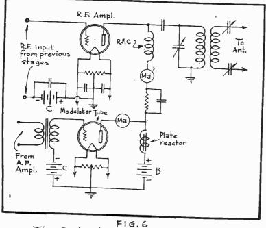
CURRENT WHICH IS DRAWN BY BOTH OF THESE TUBES MUST FLOW THROUGH THIS SAME REACTOR.
