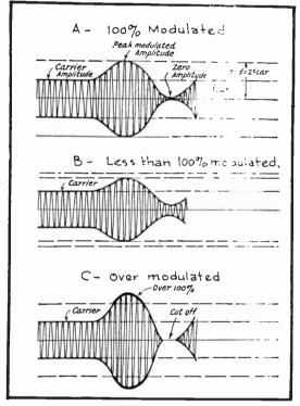
FIG. 4 Various Degrees of Modulation.
