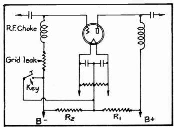
FIG.6 Blocking Grid With Bias Voltage.
