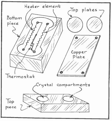
FIG. 9 Details of the Crystal Oven.
