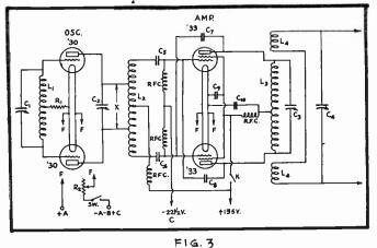
Diagram of Battery-Operated Transmitter.
