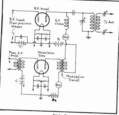
FIG. 8 Application of the Modulation Transformer.
