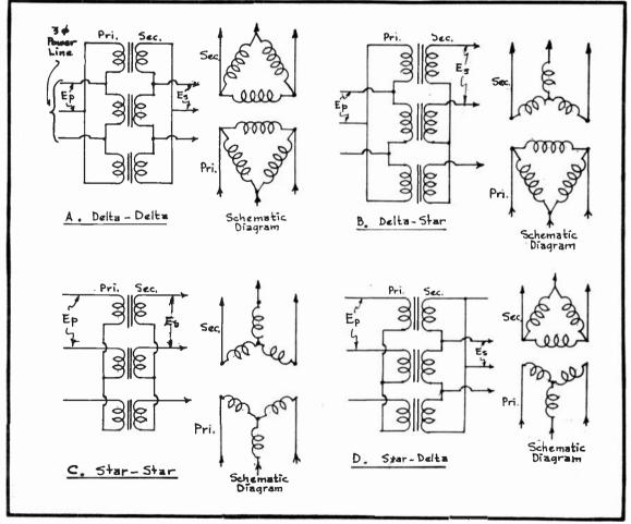
FIG. 9 Three-Phase Transformer Connections.
