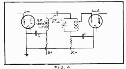
Unturned Plate - Tuned Grid Circuit.
