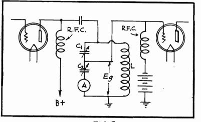
FIG.5 Another Method of Determining Grid Exitation Voltage.
