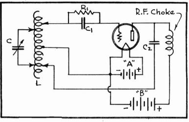
FIG. 4 Shunt-Feed Hartley Oscillator
