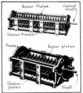
FIG.15 Typical Transmitter Tuning Condensers.
