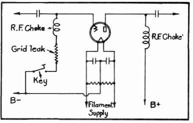
Fig.5 Grid-leak Keying.
