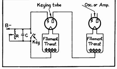
FIG.9 The Vacuum Tube Keying Method.
