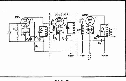
FIG.7 Low-Power Three-Tube Transmitter.
