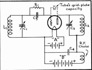
FIG.7 Tuned-Plate, Tuned-Grid Oscillator.
