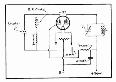
FIG. 10 Pentode Crystal Controlled Oscillator
