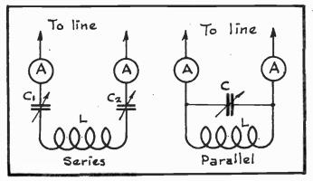
FIG. 9 Series and Parallel Feeder Tuning. ALSO IN THE ILLUSTRATION AT THE LEFT OF FIG.9. IT IS THE MORE COMMON PRACTICE TO EM-PLOY TWO TUNING CONDENSERS IN THE SERIES ARRANGEMENT AS SHOWN IN FIG.9. SERIESTUNING OF THE TRANSMISSION LINE HAS NO EFFECT ON THE CURRENT DIS TRIBUTION IN THE SYSTEM.
