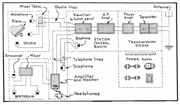
FIG. 2. Typical Arrangement of a Broadcast Station.
