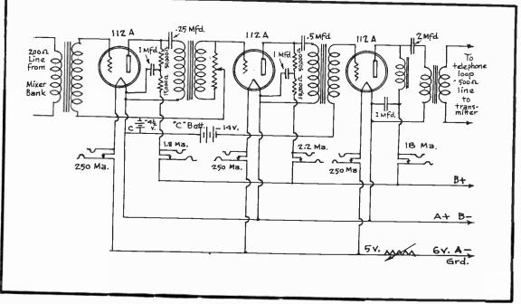
FIG. 12 The Low-level Amplifier.
