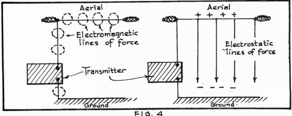
Establishing Electromagnetic and Electrostatic Fields.
