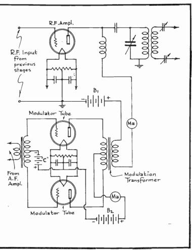
FIG: 9 Application of Push-Pull Modulator Tubes.
