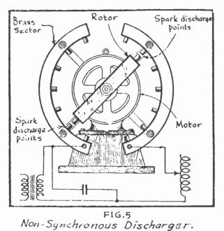
BETWEEN THE SPARK CONTACTS TO RE-MAIN & CONDUCTOR AND THIS WILLNOT PERMIT THE CONDENSER TO BECHARGED TO ITS FULL CAPACITY. THAT IS. THE CONDENSER WILL DISCHARGE AT A PO-TENTIAL LOWER THAN DESIRED AND IN STEAD OF THE OSCILLATIONS IN THE CLOSED CIRCUIT BEING STOPPEDAFTER THE AERIAL CIRCUIT HAS STARTED RA-DIATING ITS WAVES, WE FIND THAT THIS CONTINUAL ARCING ACROSS THE SPARK GAP ADDS EXTRA WAVES UPON THE ORIGINAL WAVE FORM, THEREBY PREVENTING TRANSMISSION OF "CLEAN CUT WAVES.
