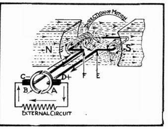
FIG. 17 Current Flow over External Circuit.
