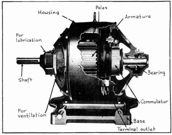
FIG. 21 A Direct Current Motor
