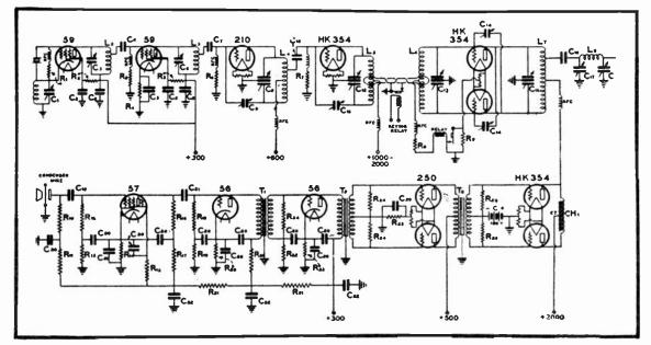
FIG. 13 The 1000-Watt Transmitter.
