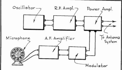
FIG. 2. Block Diagram of a Typical Radio Telephone Transmitter.
