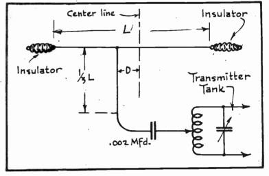
FIG.16 Single-Wire Antenna Feed.
