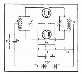
FIG. 12 The Tuned-Plate, Tuned Grid Push-Pull Oscillator.
