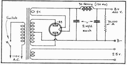
FIG. 15 Power Pack For the Pysh-Pull Transmitter.
