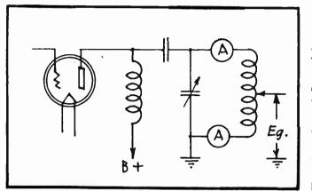
IN THE EVENT THAT THE CIRCUIT ARRANGEMENT IS SUCH AS SHOWN IN FIG. 5 AND IN WHICH THE GRID EXITATION VOLTAGE IS EQUAL TO THE VOLTAGE DEVEL-OPED ACROSS THE CONDENSER C, THEN WITH THE RADIO-FREQUEN CY AMMETER INSTALLED IN THE CIRCUIT AS SHOWN AND THE CIR-CUIT TUNED TO RESONANCE, THE GRID EXITATION VOLTAGE WILL BE FOUND FROM THE RELATION  $E_{G} = IX_{C}$  where I = THE CURR-ENT INDICATED BY THE METER AND X = THE CAPACITIVE REAC TANCE OF CONDENSER C2 AT THE
