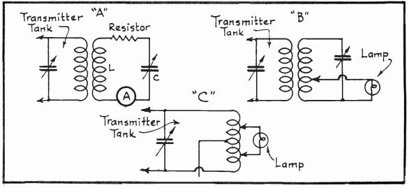
FIG. 10 Typical Dummy Antenna Circuits.
