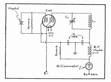
FIG. 12 A Heater-Type Pentode Crystal Oscillator.
