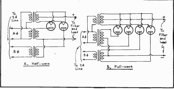
FIG. 10 Two-Phase Rectifier Circuit.
