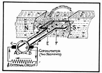
FIG. 16 The Simple D.C. Generator.
