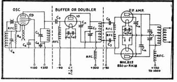
Fig.8 Transmitter With Push-Pull Power Amplifier. ENT SECTIONS HAVE ALL BEEN COMBINED TO FORM A COMPLETE TRANSMITTER UNIT. THE POWER PACKS AND KEY CIRCUITS ARENOT BEING CONSIDERED AT THE PRES-ENT TIME, SINCE THEY AREFULLY EXPLAINED IN LATER LESSONS.
