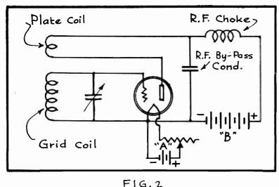
INDUCTION IN THE GRID COIL AND THE APPLICATION OF A STILL HIGHER POS-ITIVE POTENTIAL UPON THE GRID OF THE TUBE. THIS CAUSES A FURTHER IN-CREASE IN THE PLATE CUR RENT AND THEAPPLICATION OF STILL HIGHER POBITIVE POTENTIALS UPON THEGRID. THIS BUILDING-UP PROCESS CONTINUES IN THIS WAY UP TO A CERTAIN POINT AND WHICH IS DEPENDENT UPON THE CHARACTERISTICS OF THE TUBE AS WELL AS THE RESISTANCE OF THE CIRCUIT.
