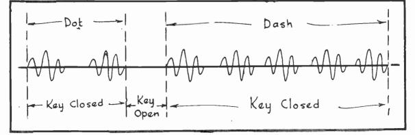
Frg. 8 Wave Radiation From Spark Transmitter.
