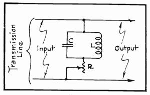
FIG.2 A Parallel-Resonance Equalizer.
