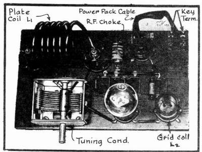
FIG.2 The One Tube Transmitter. FOR BATTERY OP-ERATION, A TYPE 30 TUBE CAN BE USED WITH 90 VOLTS ON THE PLATE OR ELSE A TYPE ~ 71Å OR AN -OIÅ WITH 180 VOLTS ON THE PLATE. FOR A STILL GREATER POWER OUTPUT AND WHEN A SUITABLE Å.C. POWER PACK IS AVAILABLE, THEN A TYPE -10 TUBE CAN BE USED WITH 500 VOLTS APPLIED TO THE PLATE.
