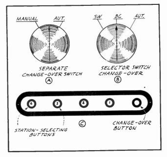
Fig. 13 Typical Change-over Methods
