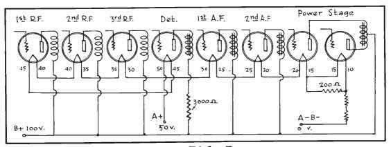
FIG. 3 Adding the Plate Circuits To the D.C. Receiver.
