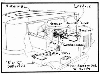
FIG. 11 Typical Auto Radio Installation.
