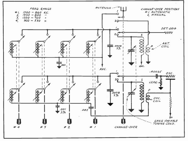
Fig. 20 Automatic Tuning System with Iron-core Coils Throughout
