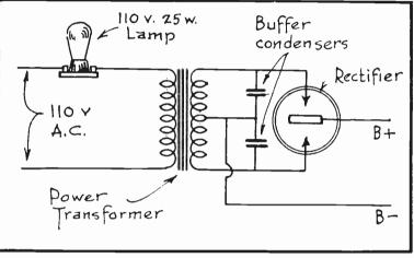
FIG.9 Checking the Secondary Circuit of the Transformer.
