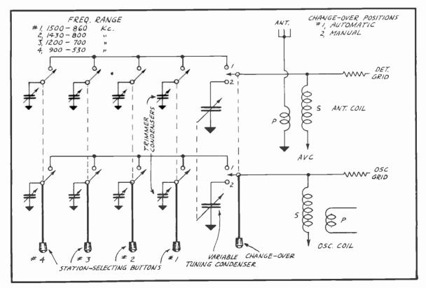
Fig. 15 Circuit Diagram of Typical Condenser-substitution System
