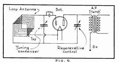
Using Regeneration With a Loop Antenna.
