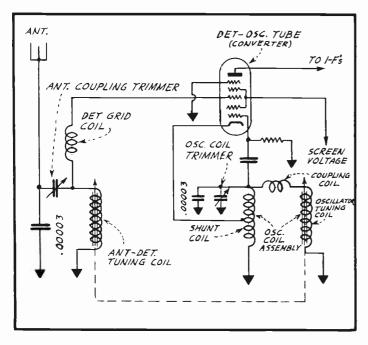
Fig. 23 Continuously-variable Permeability-tuning Circuit
