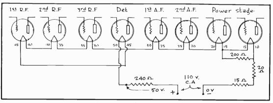
FIG. 2 Filament Connections In An Eight-Tube D.C. Receiver.
