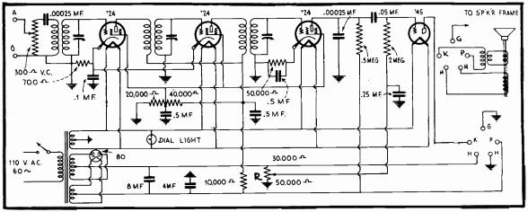
FIG. 3 A Five-Tube Midget Receiver.
