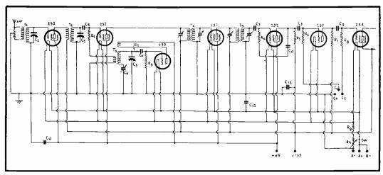
FIG. 13 Circuit Diagram of the Superheterodyne,
