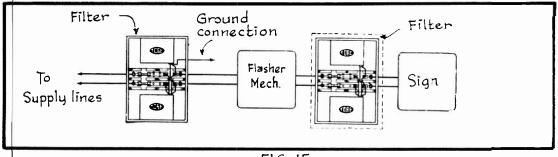
FIG. 15 Filter Installation In Flasher Sign Circuit.
