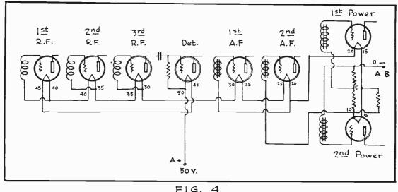
Obtaining the Grid Bias In a D.C. Receiver.
