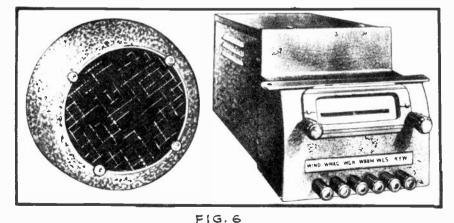
A Superheterodyne Receiver With Separate Speaker
