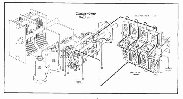
Fig. 14 Typical Condenser-substitution Tuning System
