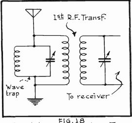
FIG. 18 A Parallel Connected Wave Trap.
