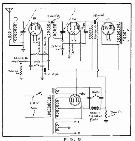
A 4 Tube Receiver with Constant-Gain Transf.
