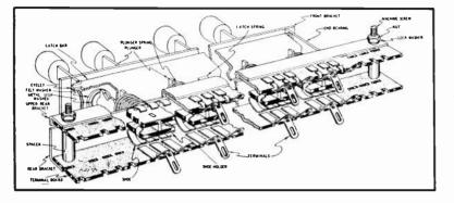
Fig. 16 Sectional View of Typical Push-Button Switch Assembly
