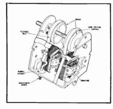
FIG. 10 THE ASSEMBLED MOTOR
