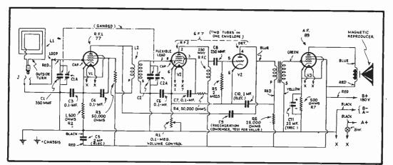
FIG. 15 Circuit Diagram of the Three-Tube Portable.
