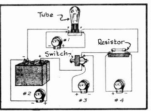
FIG. 7 Testing a Filament Circuit With a Voltmeter.
