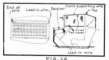
Antenna Installation On An Open Car.
