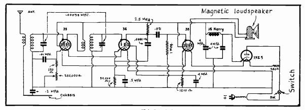
FIG. 10 Four-Tube Universal Receiver Employing a 1223 Rectifier.
