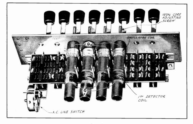
FIG. 21 Two-gang Coil and Push-button Switch Assembly
