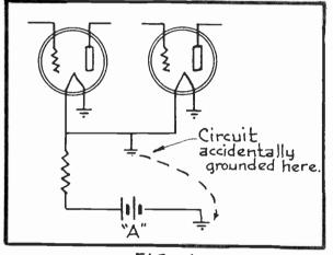
FIG. 4 A Grounded Filament Circuit.
