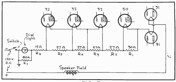
FIG. 7 The Filament Circuit.
