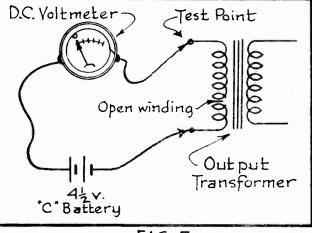
FIG. 5 Testing for an Open Transformer Winding.
