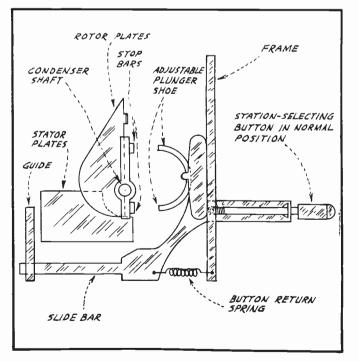
Fig. 7 Mechanical Push-button Dial Assembly
