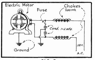
FIG. 9 Filter Connections for an Electric Motor.
