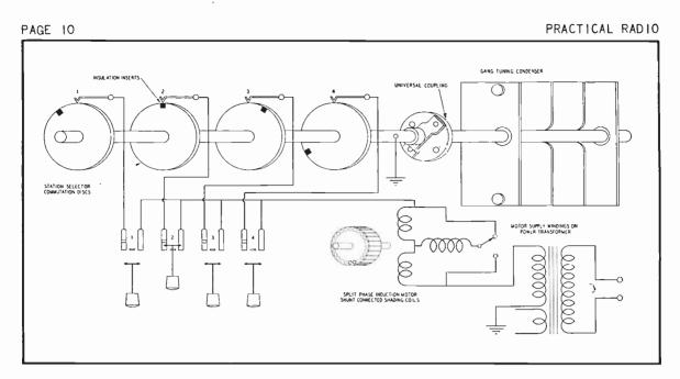
FIG. 12 Schematic Diagram of Motor-tuned System
