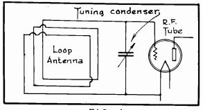
Coupling the Loop Antenna to the Input or First R.F. Tube.
