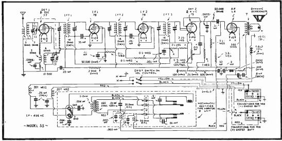
FIG. 18 A Modern Auto Receiver Circuit.
