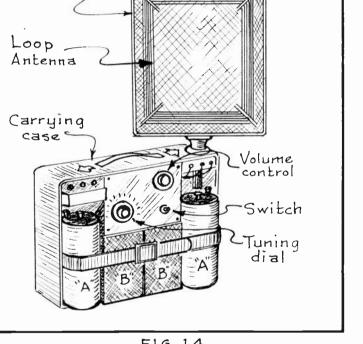
F1G.14 Portable Receiver With Loop Antenna.
