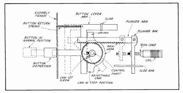
FIG. 25 CUTAWAY END-VIEW OF PERMEABILITY TUNING MECHANISM
