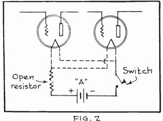
Effect of Open Filament Circuit.
