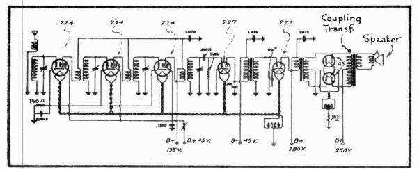
FIG. 4 An A.C. Receiver Circuit.
