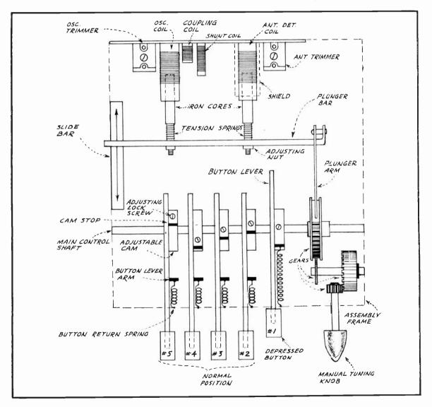
FIG. 24 Automatic Permeability-tuning Circuit
