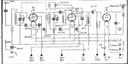
FIG. 12 A Three-Tube Regenerative fortable Receiver.
