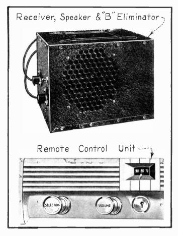
FIG. 5 Complete Auto Receiver With Remote Control
