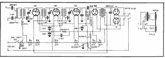
FIG. 6 The Six-Tube Screen Grid D.C. Receiver.
