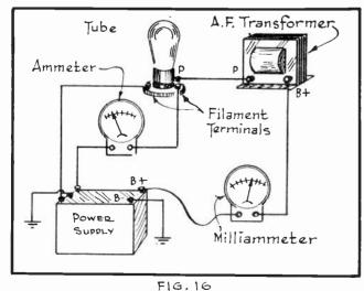
Measuring Filament and Plate Current.
