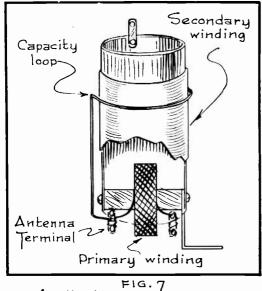
FIG. 7 Application of the Capacity loop.
