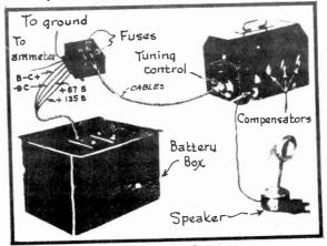
FIG. 4 Assembly Making-up The National Auto Receiver.
