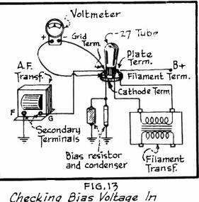
Checking Bias Voltage In Circuit Using -27 Tube.
