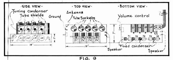
Parts Arrangement of the Receiver Circuit.
