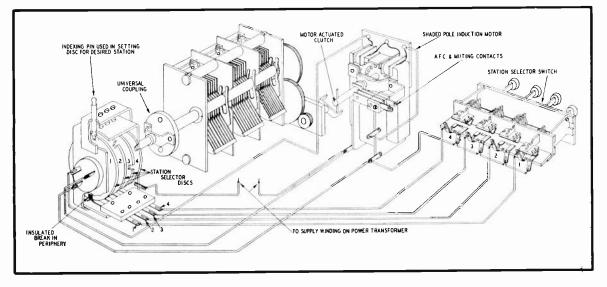
Fig. 11 Motor-driven Station-selecting System
