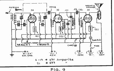
Circuit Diagram of the 3-Tube Portable.
