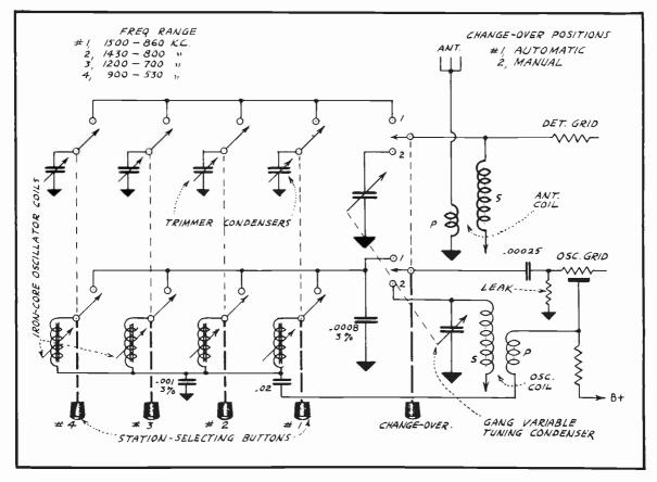
Fig. 19 Application of Iron-core Oscillator Coils
