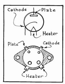
FIG.9 Symbol and Base Arrangement of the 1223. THE FACT THAT THE HEATER OF THIS TUBE IS RATED AT 12.6 VOLTS, REDUCES SOMEWHAT THE HEAT DISSIPATION REQUIRED OF THE BALLAST RESISTOR WHICH IS CONNECTED IN SERIES WITH THE HEATERS OF THE CONVENTIONAL TYPE OF UNIVERSAL RECEIVERS. THIS MEANS THAT THE RECEIVER WILL NOT BECOME QUITE SO HOT WHEN IN OPERATION. FURTHERMORE, SINCE MOST UNIVERSAL RECEIVERS REQUIRE A TOTAL PLATE CURRENT OF ABOUT 30 TO 40 MA., THE 1223 CAN MEET THIS DEMAND SATISFACTORILY.
