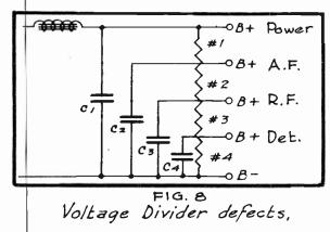
ING TUBE SOCKETS AS DETERMINED BY THE TUBE REMOVAL TEST, THEN THERE IS A POSSIBILITY OF THE TROUBLE BEING LOCATED IN THE VOLTAGE DIVIDER SYS-TEM.
