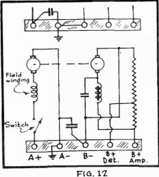
Circuit Diagram of the "Esco" Power Unit. TOR SHAFT IN A VERTICAL PLANE.
