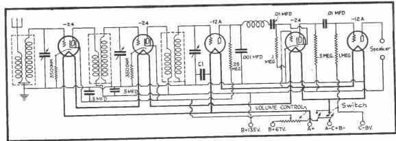
FIG. 5 Circuit Diagram of the NATIONAL Auto Receiver.
