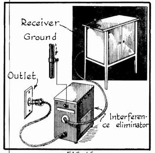
FIG.16 Connecting Interference Eliminator to A.C. Receiver.
