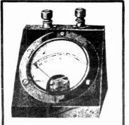
FIG.12 with O-100 M.A. Scale.
