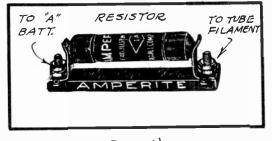
FIG. 14 A Fixed Filament Resistor
