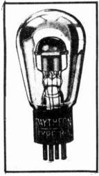
FIG.12 Full- Wave Rectifying Tube.
