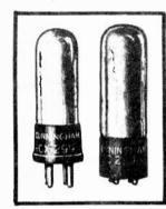
FILAMENT - A TUNGSTEN FILAMENT IS USED IN THE -99 TUBES AND IT ONLY DRAWS A CURRENT OF .063 AMPERE AT AN APPLIED FILAMENT VOLTAGE OF 3.3 VOLTS. THREE SERIES CONNECTED #6 DRY CELLS ARE GENERALLY EMPLOYED FOR THE "A" SUPPLY WHEN WIRING TUBES OF THIS TYPE. THREE DRY CELLS CONNECTED IN THIS MANNER WILL OFFER A VOLTAGE OF 4.5 VOLTS AND THIS CAN BE REDUCED TO THE REQUIRED 3.3 VOLTS BY INCLUDING A 30 TO 60 OHM RHEOSTAT 1N THE FILAMENT CIRCUIT.
