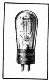
FIG. 9 *The – OOA*  OPERATION: - AS ALREADY MENTIONED, IT WILL ONLY---FUNCTION SATISFACTORILY IN CIRCUITS DESIGNED ES-PECIALLY FOR IT. A PLATE VOLTAGE OF 135 VOLTS MAY BE USED WITH A NEGATIVE GRID BIAS VOLTAGE OF 1.5 VOLTS. HOWEVER, IT IS ALSO PERMISSIBLE TO EMPLOY A PLATE VOLTAGE OF 180 VOLTS BUT UNDER THESE CON-DITIONS, THE NEGATIVE GRID BIAS VOLTAGE SHOULD BE INCREASED TO A VALUE OF 3 VOLTS. THE NORMAL PLATE CURRENT IS .2 MILLIAMPERE.
