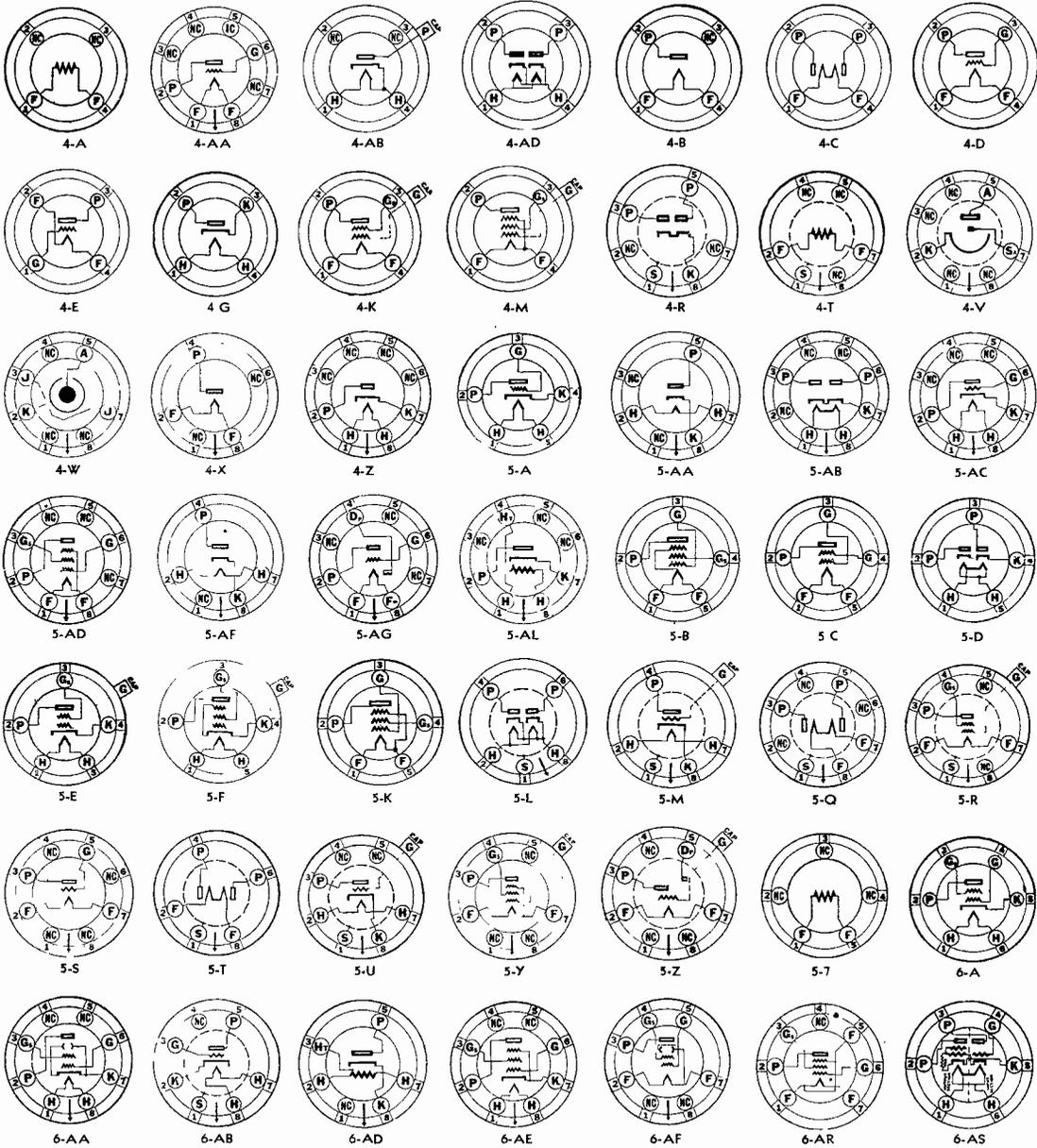
**SYMBOLS** A—Anode, A1—Anode 1, A2—Anode 2 D1—Deflector 1, D2—Deflector 2 D3—Deflector 3, D4—Deflector 4, Dp—Diode Plate, F—Filament, Fc—Filament Center, G—Control Grid, GA—Anode Grid, GM—Modulator Grid, Go—Oscillator Grid, Gs—Screen Grid, H—Heater, Hc—Heater Center, Ht—Heater Tap, IC—Internal Connection, IS—Internal Shield, J—Jumper, K—Cathode NC—No Connection, P—Plate, Rc—Ray Control, S—Metal Shell, SA—Starter Anode, Su—Suppressor Grid T—Target XS—External Shield, □—Top Cap, —>—Locating Pin
