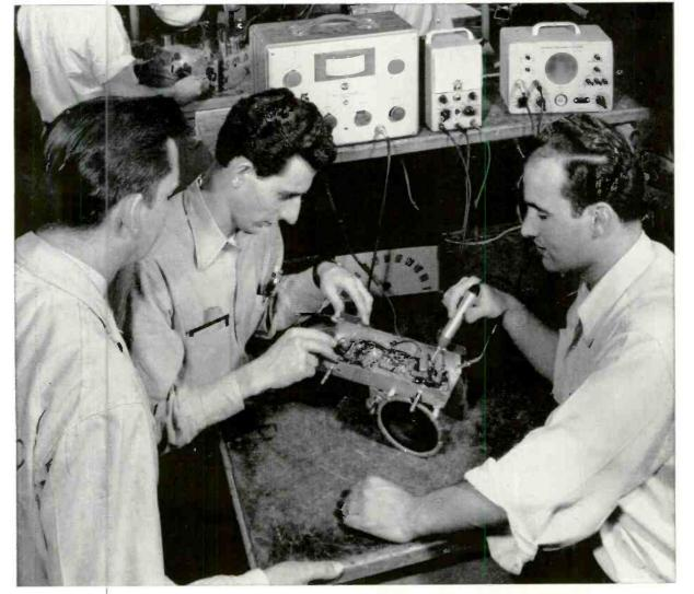
These students are getting practice in the use of Modern Test Instruments. Instructors place trouble in Receivers that are similar to the type of trouble ordinarily found by the Service Man in the field. These Receivers are then serviced by the students using Modern Test Instruments to locate the defect.
