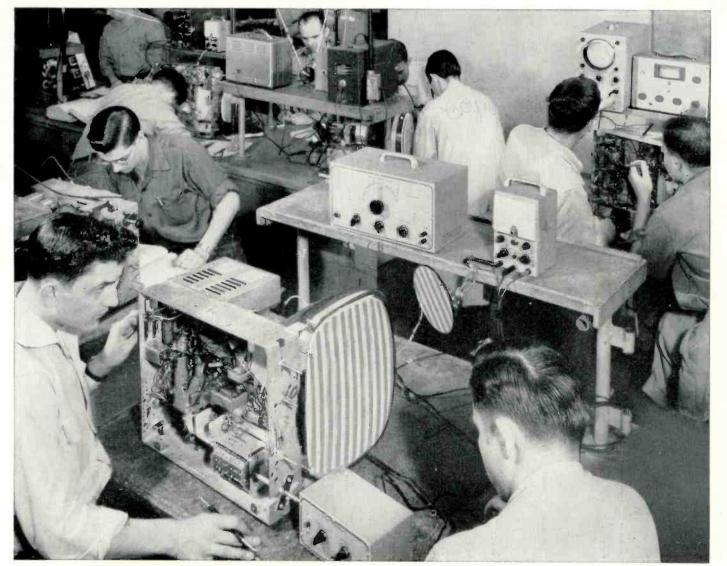
In this photo you see an instructor explaining procedures in checking linearity using a Cross Bar Generator. The students in the background are aligning and testing Receivers using various types of up-to-date testing equipment. This practical training gives the students the experience they will need out in the field.
