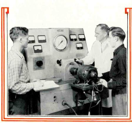
These Coyne students are testing the efficiency of a motor with a modern Dyna-mometer, a type used extensively in industry for testing A.C. and D.C. motors.
