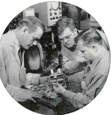
The photo above shows a section of our Television Service and Repair. This Coyne instructor is demonstrating the procedure of equipping a television receiving set to receive UHF (Ultra High Frequency) television.
