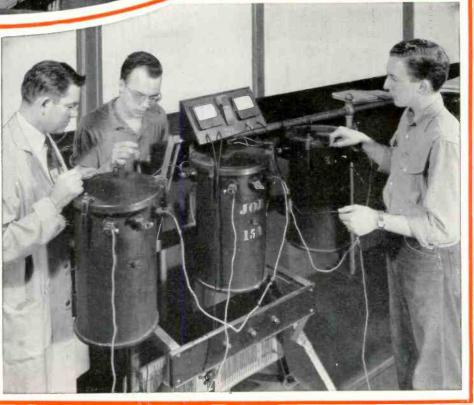
These students are connecting up a bank of power transformers for 3 phase operation, of a type commonly used in outdoor type substations.
