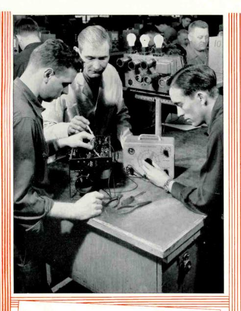
These students are building and testing Carries Current Remote Control units, with which Electrical equipment, located some distance from the operator, may be turned off or on by means of high frequency impulses sent over Alternating Current power wires.
