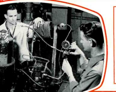
This photo shows a section of Refrigeration. These students are tracing the electrical circuits on Rotary Refrigeration units with latest types of Hermetic Analyzers. This gives them the knowledge and practice in the technique of locating faults in the electrical portion of Refrigerators. Notice the Hermetically Sealed units in glass domes in the upper left part of the photo.
