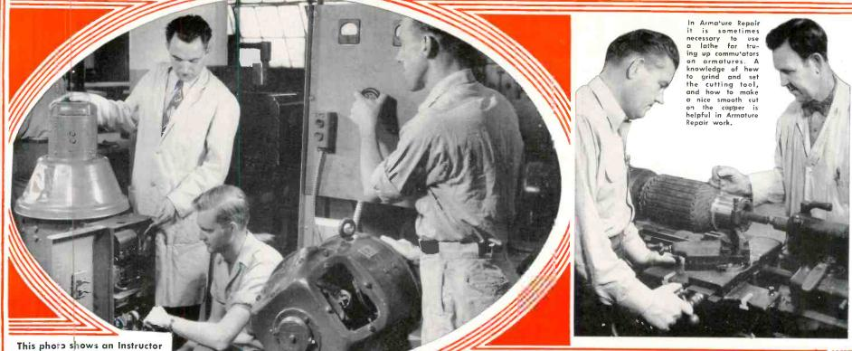
This phore shows an instructor explaining a rotating system for producing variable volt-ages used in obtaining a wide range in motor speeds. These units are used extensively in Textile, Food, Metal, Paper, Printing, Rubber, Machine Tool, Wire and Cable industries.
