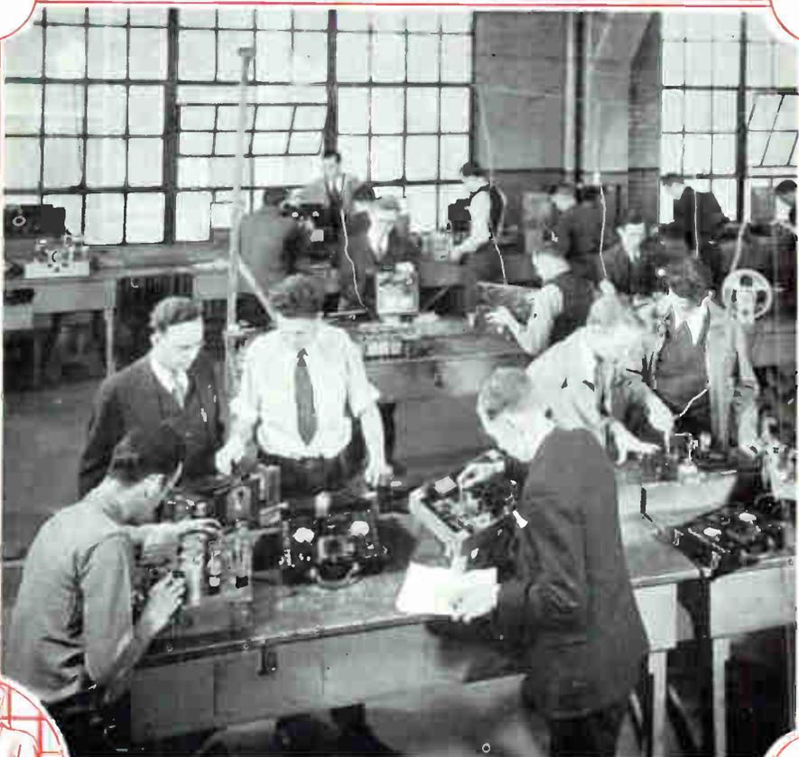
Students receiving instruction on use of modern set analyzers or trouble shooting kits. With this equipment it is easy to locate faults and defective parts in any type of set.
