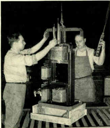
A 300-ampere 65-line welder being assembled. The transformer is already mounted in the frame and the complete reactor is being lowered into position. Hipersil type-C cores are used on both transformer and reactor.
