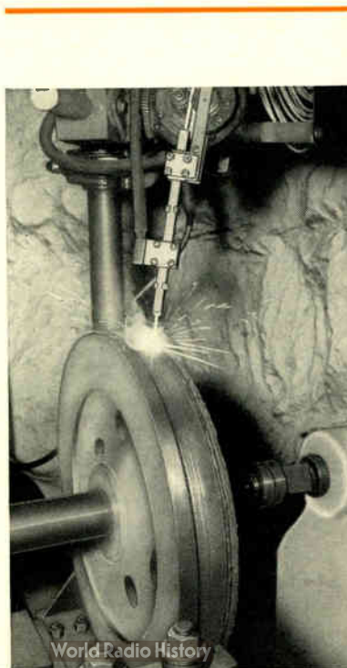
The heads for automatic arc welding—coated-electrode (two forms), bare-wire, submerged-melt, carbon-arc, and stick-feed. Rebuilding mine-car wheels by automatic welding (left) and machining.
