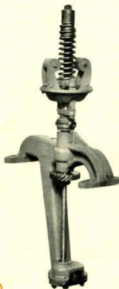
Fig. 1 (a)—Mechanism of early type flyball, gear-driven governor with oil pump mounted on a turbine shaft extension.
