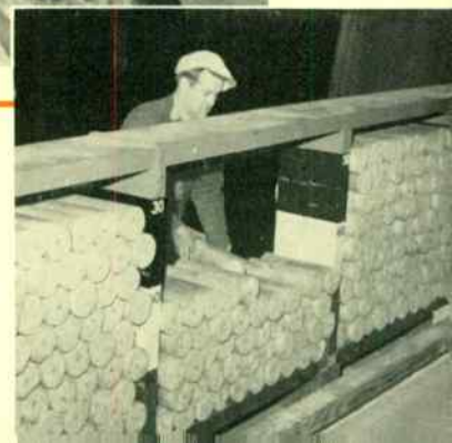
Fireplace logs are being made artificially. Sawdust and mill shavings are compressed at 50 000 psi to form dense logs four inches high by twelve long. Photos by Weyerhaeuser Timber Company.
