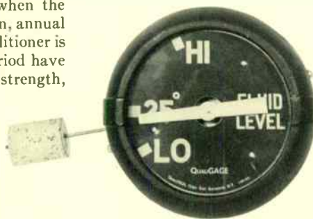
The magnetic temperature indicator (extreme left) is reset by an external magnet. At left is the liquid-level indicator. The oil conditioner (below) maintains the qualities of transformer liquids.
