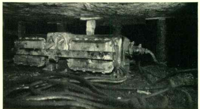
A portable sealed-tank dry-type transformer in service in a coal mine is shown above. Below is an external view of the first 500-kva, 13-kv submersible dry-type network transformer, installed in 1943. The high-voltage, single-conductor cables enter the transformer through a terminal chamber mounted on one end of the tank.
