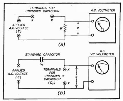
Fig. 2. Use of Voltmeter to Check Capacitance.
