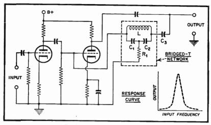
Fig. 7. Bandpass Electronic Filter.
