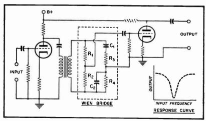
Fig. 8. Band-Suppression Electronic Filter.
