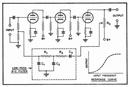
Fig. 5. High-Pass Electronic Filter.
