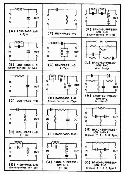
Fig. 3. Frequency-Selective Networks for Inclusion in Electronic Filters.
