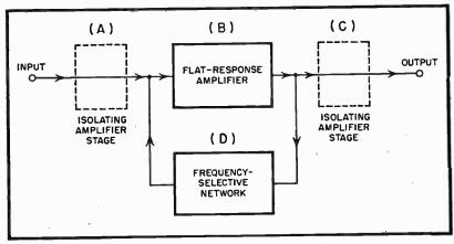
Fig. 1. Basic Feedback-Type Electronic Filter.
