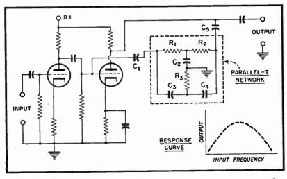
Fig. 6. Bandpass Electronic Filter.
