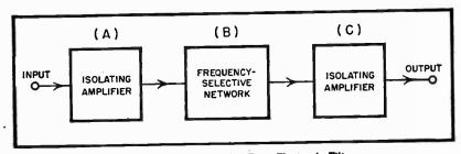
Fig. 2. Basic Transmission-Type Electronic Filter.
