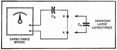
Fig. 2. Substitution measurement of large capacitance.
