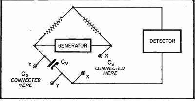
Fig. 3. Bridge adapted for substitution capacitance measurements.
