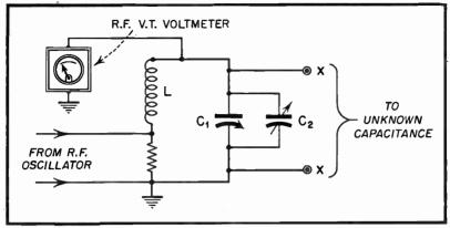
Fig. 4. Q-meter capacitance-checking circuit.
