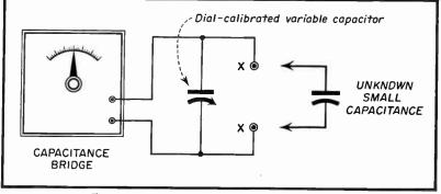
Fig. 1. Basic setup for substitution measurements.
