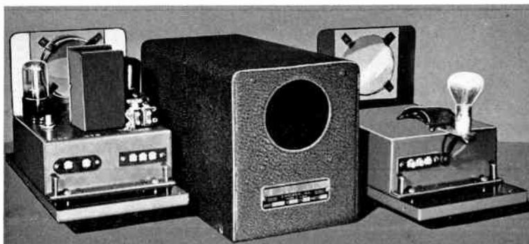
The Worner Anti-Sabotage equipment. "Black" light source (right) provides invisible light beam for the photoelectric relay at left. Interruption of beam produces audible or visible alarm.
