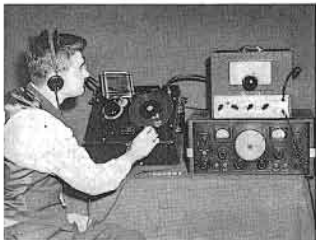
Herb Eidson measuring resistance and inductance of the ohmpac unit with an rf bridge. The rf generator and receiver is at right.
