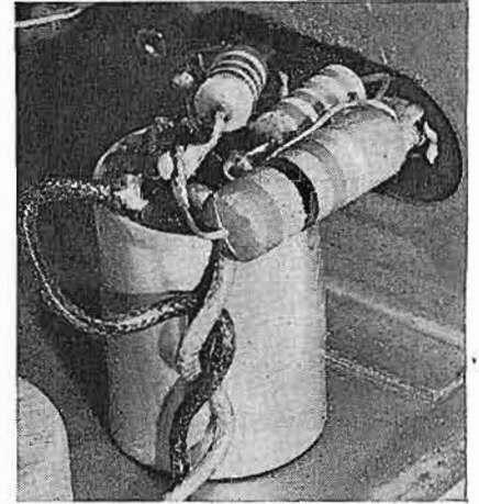
Closeup of the miniature transformer mounted in the corner of a pa amplifier next to the phono input terminal strip.
