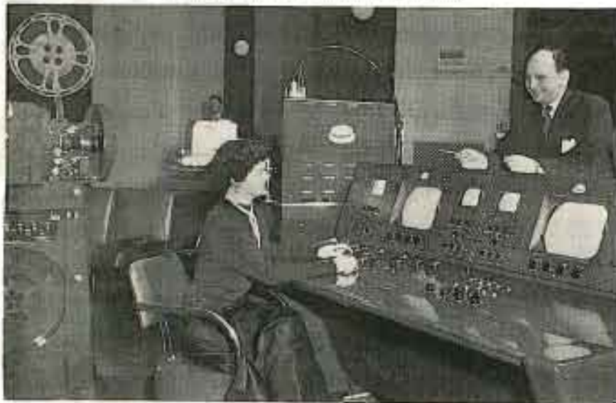
Herbert E. Taylor, Jr., of DuMont, explaining operation of the TV monitor console in the exhibition hall during the NAB Convention. Note display of TV motion picture equipment in background.
