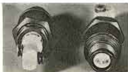
Figure 6 Two-electrode spark plugs used in 'plane tests.
