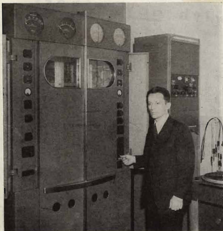
Figure 1 M. A. Honnell with the converted 1-kw f-m transmitter.
