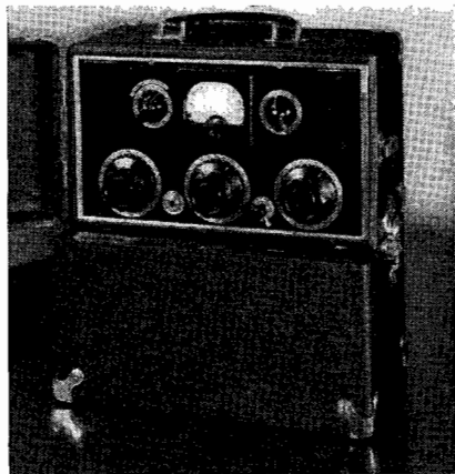
Fig. 7. The Type 2A equipment (UTC). Amplifier is in upper case, power supply in lower case.
