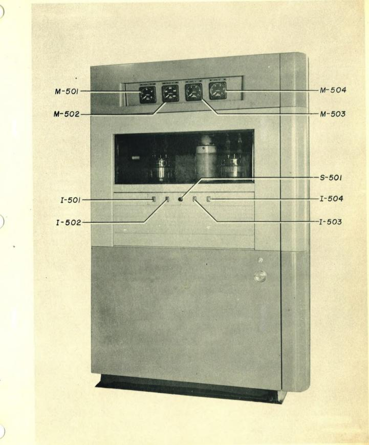
FIG. 23. Right Power Amplifier Cubicle, Front View (Photo C-12139)
