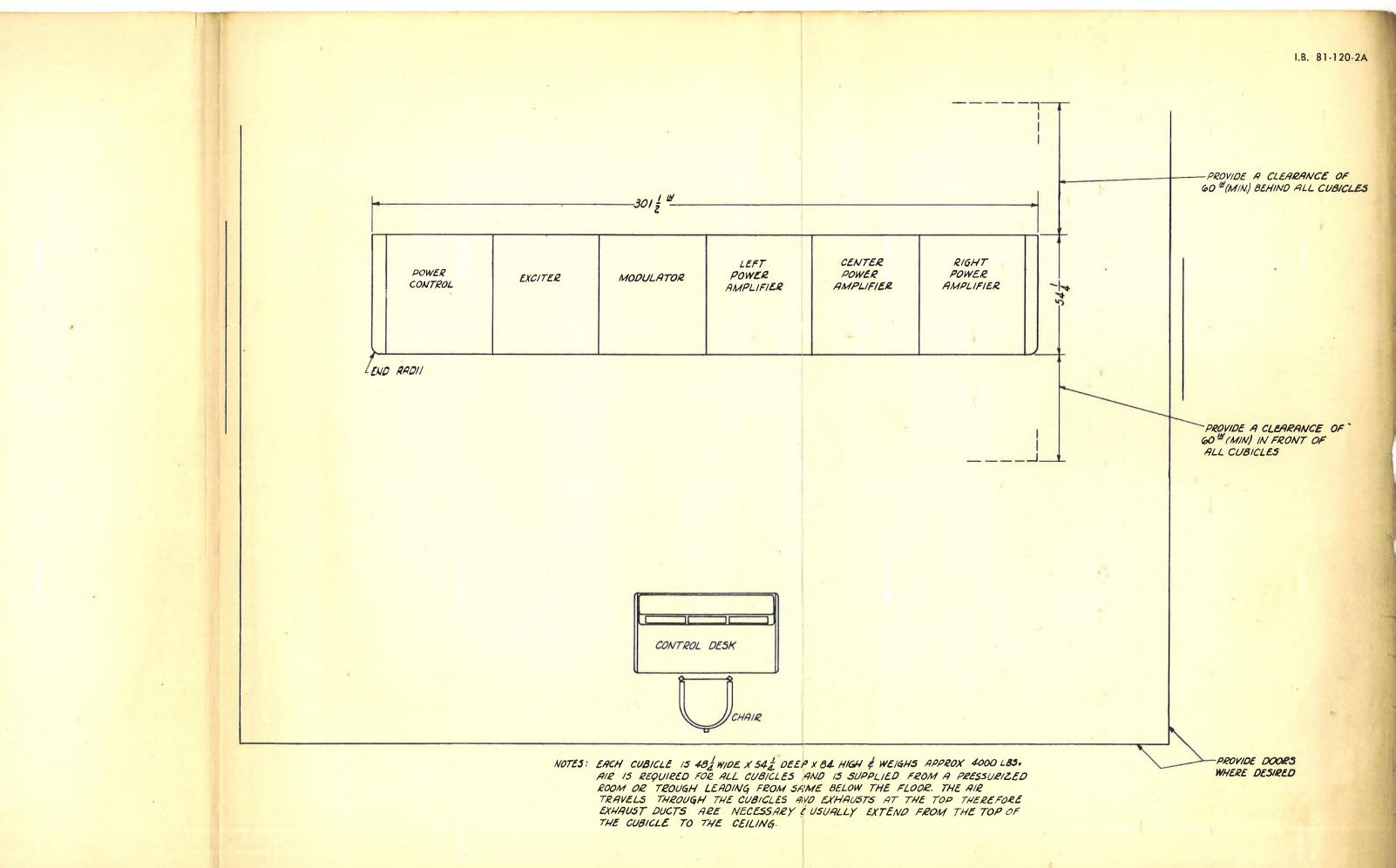
FIG. 37. Cubicle Layout—Inline (Not Walled In) (Dwg. 7720598)
