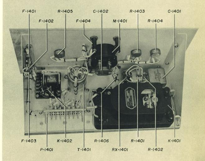
FIG. 21. Antenna Arc Interrupter Unit (Photo C-12104)
