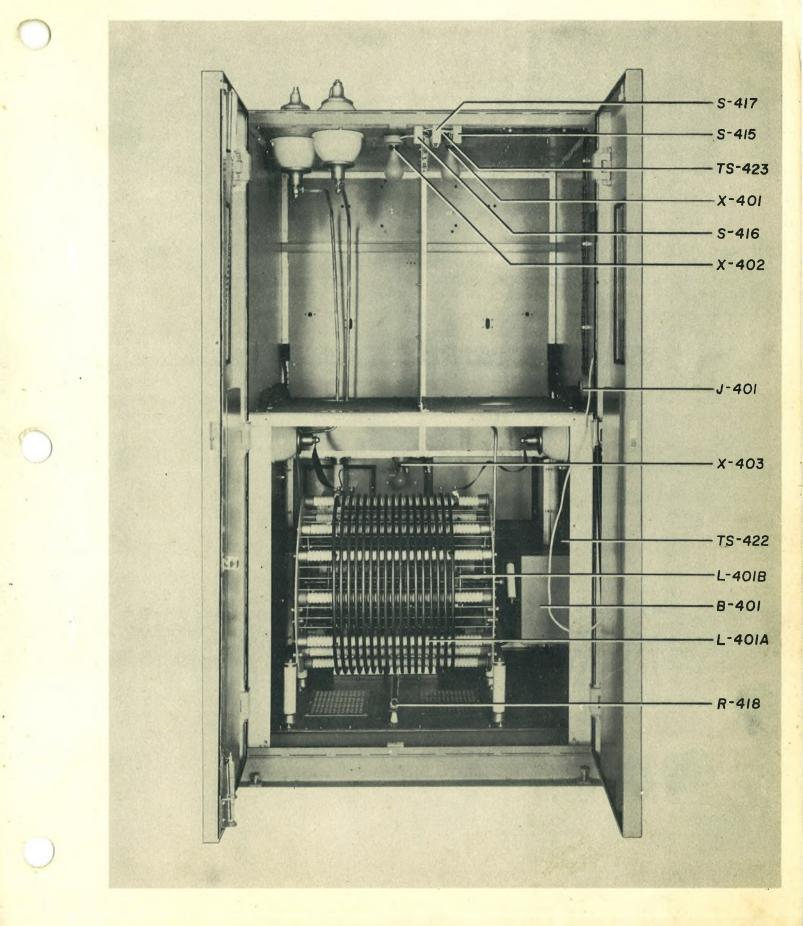
FIG. 22. Center Power Amplifier Cubicle Interior (Photo C-20278)
