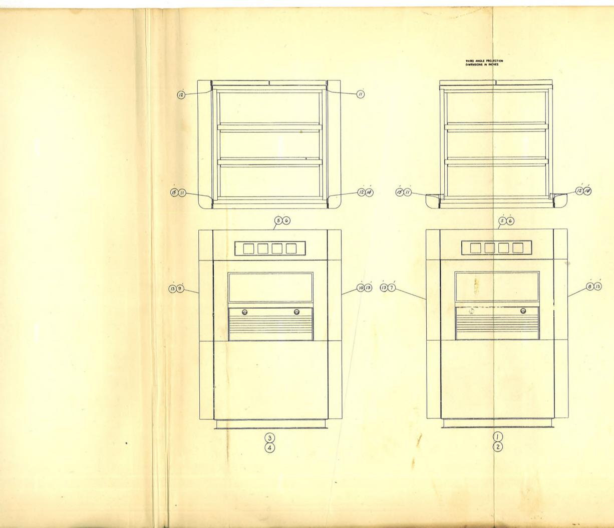
NOTES: PTS: 7, 8, 9 \$ 10 - USING PTS 11 \$ 12 AS TEMPLATES, AFTER ASSEMBLING THEM TO THE CUBICLE, DRILL AND TAP Nº 10-32 THOS. IN PTS-7, 8, 9 \$ 10, THEN ASSEMBLE USING PT.13. PTS.-11,12,146,15 ASSEMBLE TO SLOTS IN CORNER SUPPORTS OF CUBICLE.
