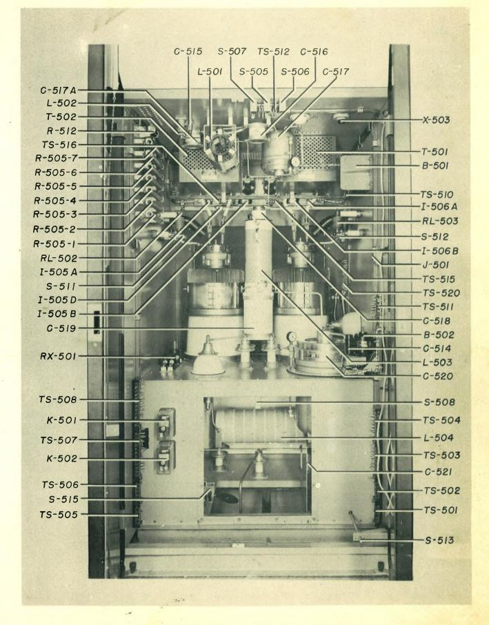
FIG. 25. Right Power Amplifier Cubicle, Interior View (Photo C-12141)
