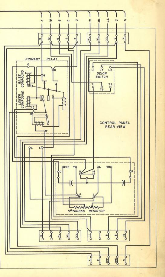
FIG. 59. Main Rectifier Regulator, Schematic Diagram (If Used) (Dwg. 7718452)
