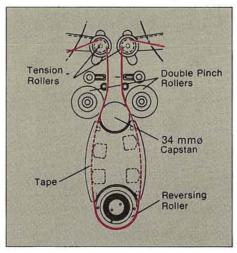
The tape in this loop is, as the name suggests, isolated from external influences such as may be imposed by the take-up reel or the supply reel. It is within
