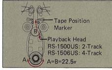
To aid in editing, the tape is put into contact with the playback heads in the fast-forward and rewind modes. By means of blip-counts, one can quickly locate a desired section of tape.
