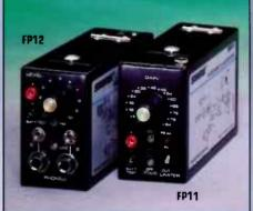
**FP11** The FP11 Mic-to-Line amplifier provides up to 84 dB of additional gain in fourteen 6 dB steps for boosting microphone and auxiliary level devices to line level. This compact amplifier includes: a transformer-balanced XLR input and output; switchable peak limiter; peak/limiter LED indicator; aux level mini-phone jack input; balanced line-level binding post output; and removable belt clip. Powered by standard 9-volt battery.
