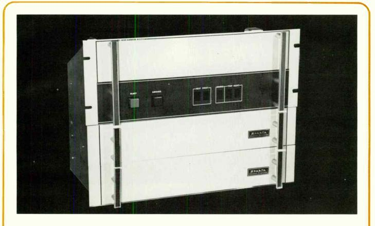
The RS4100 Random Access differs in some fundamentals from the RS250, but basically accomplishes double the work in less than double the space. The RS4100 controls four Carousels (96 tape cartridges) or a total of 100 events. Like the RS250, the 4100 presents the 96 tape cartridges it can control as a single audio source to the Model 1052 Program Controller. Besides being used with Models RS124 or 224 Carousels in systems using the Model 1052, it can be added to an existing system to upgrade it.
