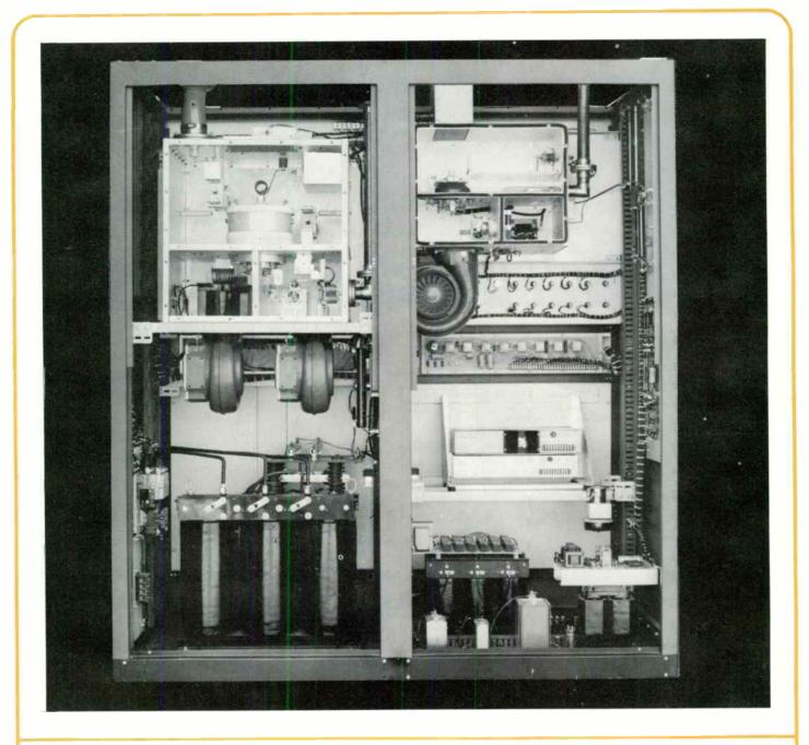
The above picture shows the roll-out high voltage power supply which is contained within the main transmitter housing. There are four heavy-duty "dolly" type casters upon which the power supply rolls. Maintenance is a simple task in the 625A FM Transmitter because of well planned features such as these and by ease of accessibility through either front or rear doors.
