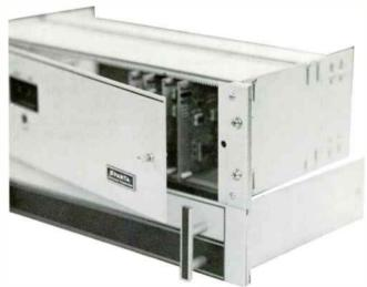
One RS250 and two RS124 Carousels are most commonly supplied with interconnecting cables cut for mounting the Random Access directly above adjacent Carousels. This combination, unmounted, is available as the SPARTAMATE "SPOT BANK" package for addition to existing SPARTAMATION or other automation systems. The RS250 takes 8¾" of rack space.
