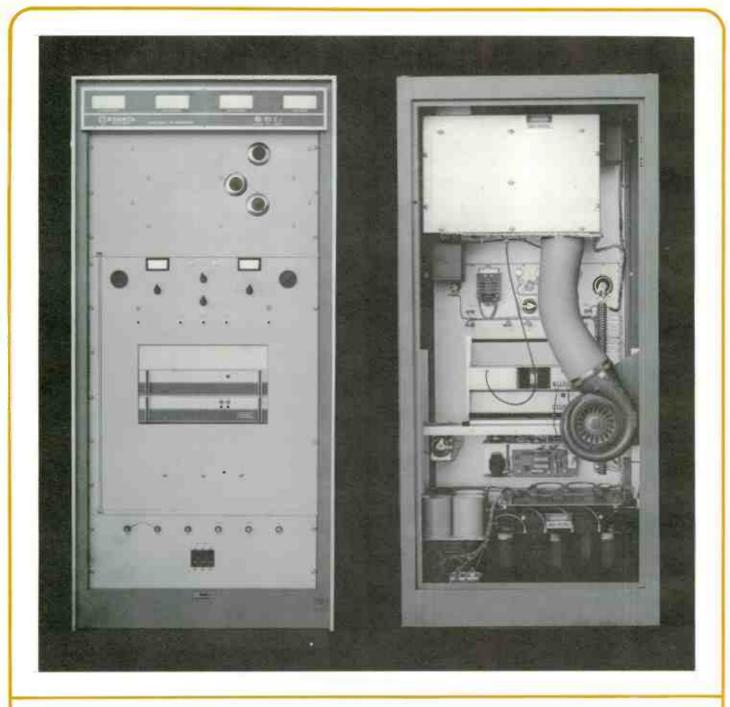
The SPARTA Model 605A is the only FM transmitter designed for primary operation at 5,000 watts! It's tube type, cabinet size and circuitry were designed to perform most economically at this power. And it's the smallest self-contained 5 kw FM available!
