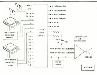
Functional Diagram for the ASC-305B Stereo Studio Control and Remote Unit
