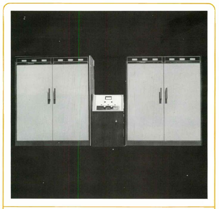
The Sparta Model 725 utilizes a unique ferrite combiner to parallel the outputs of two 12.5 kw transmitters for a power output of 25 kw. Except for a common RF drive unit, each transmitter maintains its individuality and can be operated independently of the other ... either into the built-in load or the antenna system. Automatic operation of the changeover is available, if desired.
