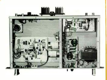
The Model 680 FM Exciter uses the most recent advances known in RF design. Its features include Strip Line Circuitry, Automatic Carrier Balance and an ovenless Digital AFC control circuit;
