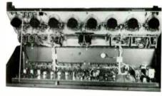
Front panel lifts for easy access to circuit modules.
