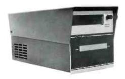
The compact CENTURY SERIES playback module is shown here with its single Fliptop cover for table-top use. The Stop/Start 'Touchbar' control is illuminated for positive control room identification. A soft but definite rose-red glow lights the left side of the bar when the module is at standby or ready. When running, the right side glows lime-green and the red light is out. Fliptop covers have a non-glare 'orange peel' textured Bittersweet Orange finish.
