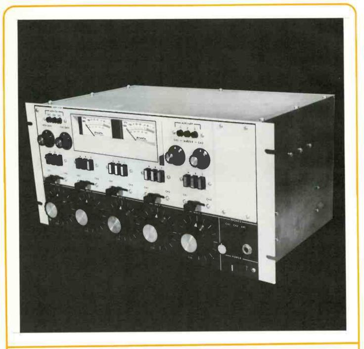
Fifteen inputs with two separate output channels! That's capability. And the new A-16R has it. It's a dual channel audio console. The A-16R easily handles several studios at once. Or with its independent VU meters you can air your program while doing production work. TV, CCTV and CATV stations are using the A-16R.
