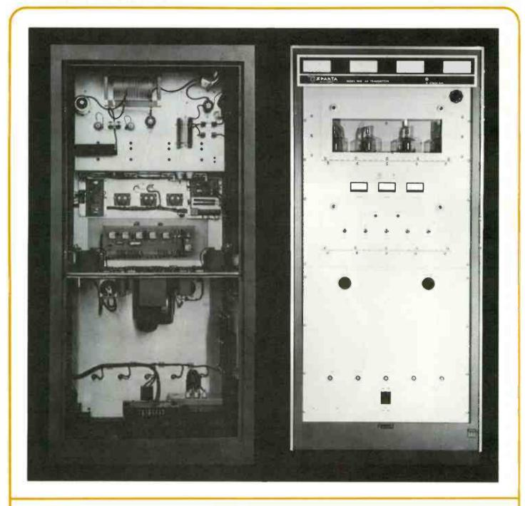
The simple straightforward engineering design of the new Model 701B is illustrated even in the classically simple layout of the front panel. The panel below the tubes and meters drops down for easy access. On its face are the "tally lights," which tell the engineer at a glance where his overload problem may have occurred, even though the automatic reset has returned the transmitter to the air.
