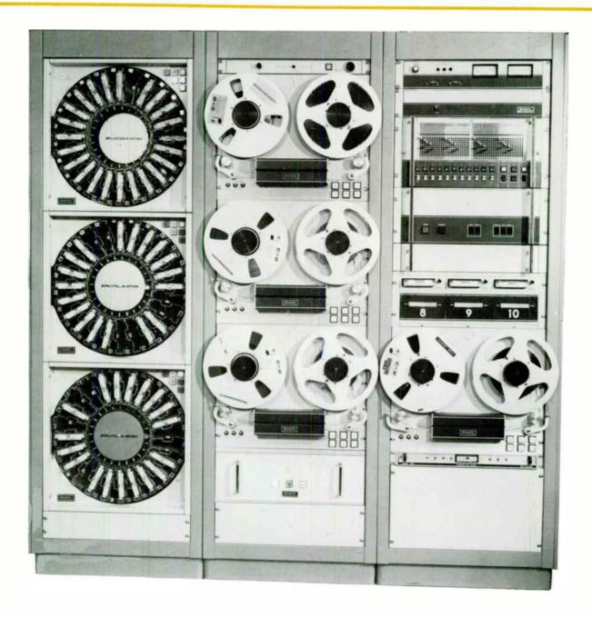
COMMERCIALS: RS-124 or 224 Carousels<sup>T.M.</sup> assure quality playback of stereo or mono accouncements. Each Carousel holds 24 cartridges. Each cartridge can hold several spots that play in rotation — up to 10½ minutes per cartridge. Each time a cartridge is played, the next announcement is readied by the Cartridge Random Access.
