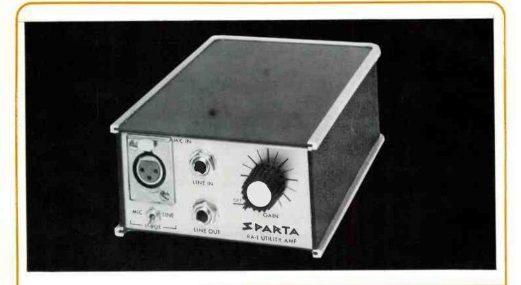
The RA-1 is a general purpose amplifier for use as a microphone preamplifier, a line booster amplifier or a remote station amplifier. As a microphone preamplifier, up to 65 db of gain is provided; as a line amplifier it will furnish up to 30 db of gain. In both applications, the output level is 10 dbm nominal into 600 ohms with a minimum of 12 db additional head-room.
