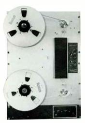
The Corinthian deck provides long periods of unattended SPARTAMATION operation. Foil reversing ensures maximum use of tapes. The capstan is direct drive with dual speed hysteresis synchronous motor. A front panel level control is screwdriver adjusted. Amplifiers are plug-in.
