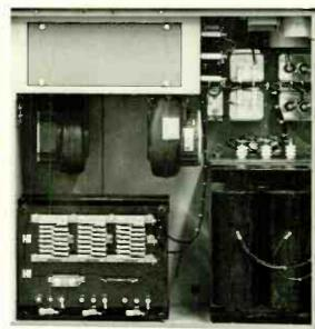
The outward appearance of both the Model 705 and 710 AM Transmitters is very similar. The metering and control functions in the 705 and 710 are identical. The difference is shown directly above. The power supply, modulation transformer and reactor are larger in the 710.
