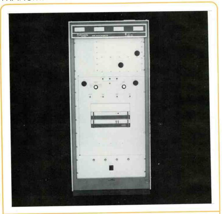
The SPARTA 602A Transmitter with a three bay circularly polarized antenna makes up the most economical package for full power Class A broadcasting. Its 2500 watts along with the standard 1.5 gain of a 3 bay circularly polarized antenna easily delivers the maximum 3000 watts ERP. Competitive transmitters require four bays to accomplish the same thing.
