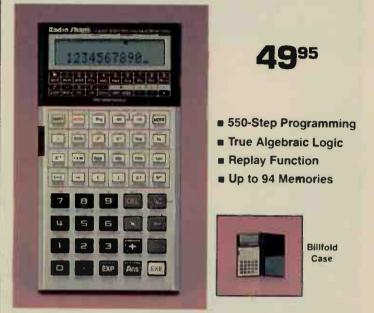
Radio Shack EC-4020. Our most powerful programmable calculator! Features three operation modes and four calculation modes. Stores up to 10 programs. Alphabetic dot-matrix display, base calculations/conversions. logical operations. Has a 12-digit mantissa and 2-digit exponent. Auto power-off. With RS-CR2032 batteries, 131-page manual. 53/16 x 23/4 x 3/8"
