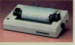
DMP 105, Another Radio Shack price breakthrough! Ideal for data processing and general-purpose use. Produces crisp 8 x 9 characters on an 8" line. Bidirectional—prints 80 upper and lowercase characters per line at 43 lines per minute (10 characters per inch). Features elongated and condensed modes. Parallel and Color Computer-compatible serial interfaces. UL listed
