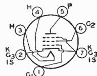
seven-contact socket and may be mounted in any position. Except for a slightly higher transconductance, this type is similar electrically to type 6AG5. Heater volts (ac/dc), 6.3; amperes, 0.3. For heater and cathode considerations, refer to type 6AV6.
