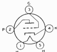
Glass type used as voltage amplifier or detector in radio receivers. Outline 32, OUTLINES SECTION. Tube requires five-contact socket. Heater volts (ac/dc), 6.3; amperes, 0.3. Characteristics as class A<sub>1</sub> amplifier: plate volts, 250 *max*; grid volts, -13.5; plate ma., 5; plate resistance, 9500 ohms; transconductance, 1450  $\mu$ mhos. For typical operation as a resistance-
