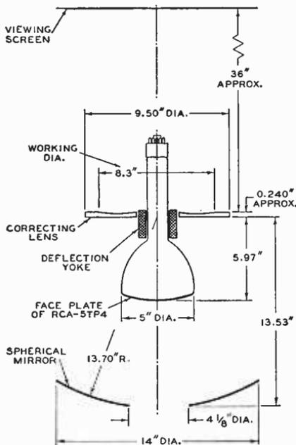
A typical reflective optical system for use with the 5TP4 is illustrated in the accompanying sketch. It consists of a spherical collecting mirror and a correcting lens located at the center of curvature of the mirror. The illustration also shows the location of the face plate of the 5TP4 and the location of the viewing screen with respect to the mirror and the correcting lens.
