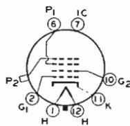
silicate type. Highlight brightness of the projected picture is about 15 foot-lamberts when the 5TP4 is operated at 27 kilovolts. Utilizes electrostatic focusing and magnetic deflection. Has deflection angle of about 50°.
