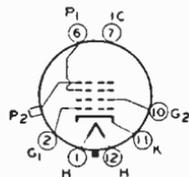
emission characteristic of this phosphor, refer to type 12LP4-A. The 7DP4 has electrostatic focus and magnetic deflection to provide a rectangular picture with rounded corners about 5½ x 4 inches or a rounded-end picture 6¾ x 4¾ inches. Has a deflection angle of approximately 50°. Tube requires duodecal twelve-contact socket and may be mounted in any position. Outline 45, OUTLINES SECTION. For installation and handling considerations, refer to ELECTRON TUBE INSTALLATION SECTION.
