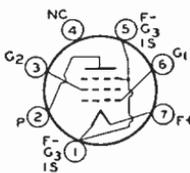
Miniature type used in light-weight, compact, portable, battery-operated receivers as rf or if amplifier. Because of internal shielding feature, an external bulb shield is not needed, but socket shielding is essential if minimum grid-No.1-to-plate capacitance is to be obtained. Outline 12, OUTLINES SECTION. Tube requires miniature seven-contact socket and may be mounted in any position. For curve of average plate characteristics, see next page. For filament considerations, refer to type 1U4.
