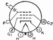
plate. The face plate of the 12LP4-A is made of RCA "Filterglass" to provide increased contrast. Type 12LP4-A supersedes type 12LP4. Both types have a deflection angle of approximately 57°, contain an ion-trap electron gun requiring an external, double-field magnet, and utilize magnetic focus and magnetic deflection to provide a rounded-end picture 11 3/8 x 8 1/2 inches or a rectangular picture with rounded corners about 10 x 7 1/2 inches.
