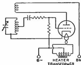
produced by electrostatic or electromagnetic coupling between the grid and plate circuits. When sufficient energy is fed back to more than compensate for the loss in the grid circuit, the tube will oscillate. The action consists of regular surges of power between the plate and the grid circuit at a frequency dependent on the circuit constants of inductance and capacitance. By proper choice of these values, the frequency may be adjusted over a very wide range.
