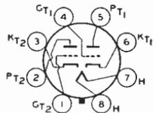
any position. Except for the common heater, each triode unit is independent of the other. For typical operation as phase inverter or resistance-coupled amplifier, refer to Chart 7, **RESISTANCE-COUPLED AMPLIFIER SECTION**. For heater and cathode considerations, refer to type 6AV6.
