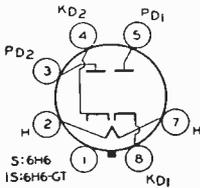
Metal type 6H6 and glass-octal type 6H6-GT are used as detectors, low-voltage rectifiers, and avc tubes. Except for the common heater, the two diode units are independent of
