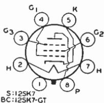
(ac/dc), 12.6; amperes, 0.15. Except for heater rating, type 12SK7 is identical with metal type 6SK7, and type 12SK7-GT is identical with glass-octal type 6SK7-GT.
