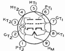
Outline 13, OUTLINES SECTION. Tube requires noval nine-contact socket and may be mounted in any position. Its characteristics are similar to glass-octal type 6SN7-GT. Each triode unit is independent of the other except for the common heater. For typical operation as a resistance-coupled amplifier, refer to Chart 10, RESISTANCE-COUPLED AMPLIFIER SECTION.
