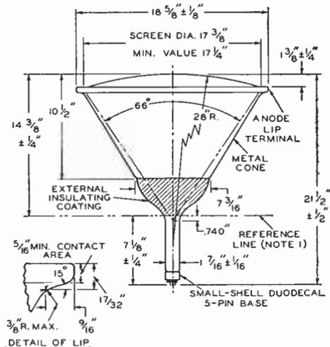
NOTE 1: Reference line s determined by position where hinged gauge  $1.500 \pm .003 \text{---} .000$ " I.D. and 2" long will rest on bulb cone.
