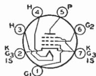
OUTLINES SECTION. Tube requires miniature seven-contact socket and may be mounted in any position. For heater and cathode considerations, refer to type 6AV6.
