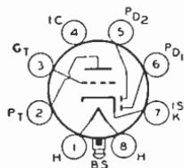
Glass lock-in type used as combined detector, amplifier, and avc tube. Outline 14, OUTLINES SECTION. Tube requires lock-in socket. Heater volts (ac/dc), 6.3; amperes, 0.3. Except for interelectrode capacitances, this type is the same electrically as metal type 6SQ7.
