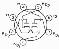
Resonant frequency of each unit is approximately 700 megacycles per second. Outline 9, OUTLINES SECTION. Tube requires miniature seven-contact socket and may be mounted in any position. For heater and cathode considerations, refer to type 6AV6.
