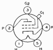
conductance, 1050  $\mu$ hos; plate ma., 4; grid-No.2 ma., 1.7 *max*. This type is used principally for renewal purposes.
