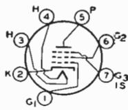
features very high transconductance combined with low interelectrode capacitance values, and is provided with separate base pins for grid No.3 and the cathode to permit the use of an unbypassed cathode resistor to minimize the effects of regeneration. Outline 12, OUTLINES SECTION. Tube requires miniature seven-contact socket and may be mounted in any position. For heater and cathode considerations, refer to type 6AV6.
