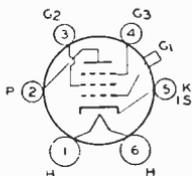
Glass type used in rf and if stages of radio receivers, particularly those employing avc. Outline 34, OUTLINES SECTION. Tube requires six-contact socket. Heater volts (ac/dc), 6.3; amperes, 0.3. Except for capacitances, this type is identical electrically with metal type 6K7. Type 78 is used principally for renewal purposes.
