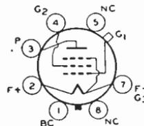
Glass octal type used as rf or if amplifier in battery-operated receivers. Outline 23, OUTLINES SECTION. Tube requires octal socket and may be mounted in any position. When used
