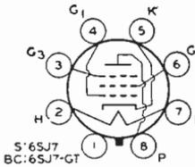
Metal type 6SJ7 and glass-octal type 6SJ7-GT are used as rf amplifiers and biased detectors. As a detector, either type is capable of delivering large audio-frequency output voltage with relatively small input voltage.
