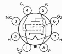
volts, 150; grid-No. 1 volts, -3; peak af grid-No. 1 volts, 3; zero-signal plate ma., 30; maximum-signal plate ma., 30.5; zero-signal grid-No. 2 ma., 7; maximum-signal grid-No. 2 ma., 9; plate resistance, 130000 ohms; transconductance, 11000  $\mu$ mhos; load resistance 10000 ohms; total harmonic distortion, 7 per cent; maximum-signal output watts, 3.
