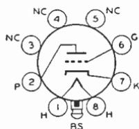
Glass lock-in type used in resistance-coupled amplifier circuits. Outline 14, OUTLINES SECTION. Tube requires lock-in socket. Heater volts (ac/dc), 6.3; amperes, 0.3. Except for interelectrode capacitances, this type has the same maximum ratings and characteristics as metal types 6F5 and 6SF5.
