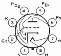
trically as type 6AT6. Outline 3, OUTLINES SECTION. Tube requires octal socket and may be mounted in any position. Heater volts (ac/dc), 6.3; amperes, 0.15. Direct interelectrode capacitances of triode unit (shell connected to cathode): grid to plate, 1.1  $\mu$ f; input, 2.4  $\mu$ f; output, 2.8  $\mu$ f. For diode operation curves, refer to type 6SQ7.
