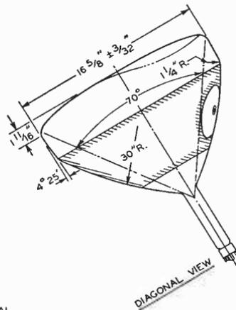
NOTE 1: With tube neck inserted through flared end of reference-line gauge (see page 291) and with tube seated in gauge, the reference line is determined by the intersection of the plane CC' of the gauge with the glass funnel.
