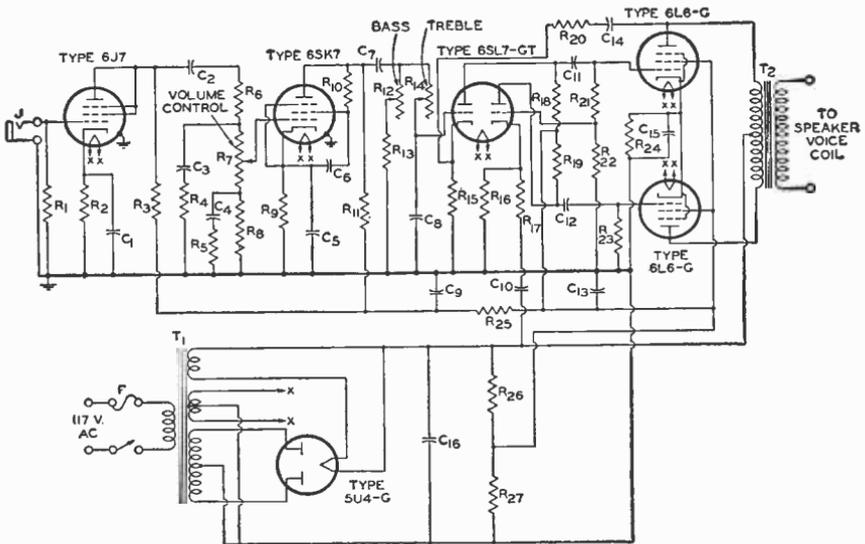
C<sub>1</sub> C<sub>5</sub> C<sub>15</sub>=20  $\mu$ f, electrolytic, 25 v.
