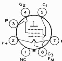
series filament arrangement, filament voltage is applied between pins 2 and 7. For parallel filament arrangement, filament voltage is applied between pin 8 and pins 2 and 7 connected together. For additional filament considerations, refer to type 3V4 and ELECTRON TUBE INSTALLATION SECTION.
