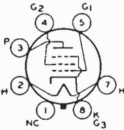
Glass octal type used in output stage of radio receivers where moderate power output is required. This type is economical because of its low plate-power requirements and low heater current. Outline 31, OUTLINES SECTION. Tube requires octal socket. Except for interelectrode capacitances and a plate resistance of 175000 ohms, this type is electrically identical with type 6AK6. Heater volts (ac/dc), 6.3; amperes, 0.15.
