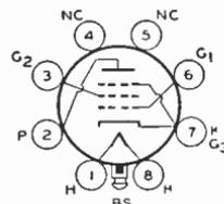
Glass lock-in type used in output stage of radio receivers. Outline 19, OUTLINES SECTION. Tube requires lock-in socket. Heater volts (ac/dc), 6.3; amperes, 0.4. Except for interelectrode capacitances, this type is the same electrically as glass-octal type 6K6-GT.
