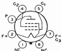
6.5; grid-No.2 ma. (zero-signal), 0.8; grid-No.2 ma. (maximum signal), 1.5; plate resistance, 0.25 megohm; transconductance, 1150  $\mu\text{mhos}$ ; load resistance, 14000 ohms; total harmonic distortion, 7.5 per cent; output watts, 0.17.
