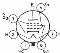
Tube requires octal socket. Vertical tube mounting is preferred but horizontal operation is permissible if pins No.2 and 7 are in vertical plane.
