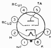
trode supply volts, 250 *max*; peak heater-cathode volts, 90 *max*. Typical operation: target volts, 250; target ma., 2.2; series resistor, 1 megohm; ray-control electrode volts (approx. for 0° shadow angle), 160; ray-control electrode volts (approx. for 90° shadow angle), 0.
