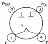
but horizontal mounting is permissible if pins 1 and 4 are in horizontal plane. Filament volts (ac), 5.0; amperes, 3.0. For maximum ratings, typical operation, and curves, refer to type 5U4-G.
