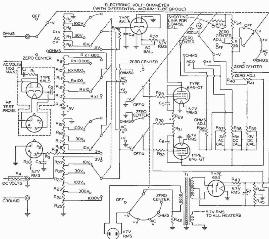
C<sub>1</sub> C<sub>3</sub> = 0.05  $\mu$ f, oil-filled, 600 v.
