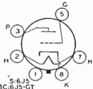
high amplification factor. Outlines 3 and 24, respectively, OUTLINES SECTION. Tubes require octal socket and may be mounted in any position. For heater and cathode considerations, refer to type 6AV6. For typical operation as a resistance-coupled amplifier, refer to Chart 13, RESISTANCE-COUPLED AMPLIFIER SECTION.
