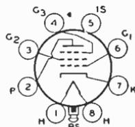
max watt; grid No.1 volts, -3; grid No.3 connected to cathode at socket; plate resistance, greater than 1 megohm; transconductance, 1575 μmhos; plate ma., 2.2; grid-No.2 ma., 0.7. Within the limits of its maximum ratings, this type is similar in performance to metal types 6SJ7 and 12SJ7.
