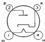
Glass type used in power supply of ac/dc receivers. Outline 32, OUTLINES SECTION. Tube requires four-contact socket and may be mounted in any position. It is especially important that this tube, like other power-handling tubes, should be adequately ventilated. Use of capacitor-input filter recommended in order to obtain as high a dc output voltage as
