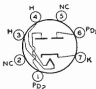
Miniature type used in power supply of automobile and ac-operated radio receivers. Equivalent in performance to larger types 6X5 and 6X5-GT.
