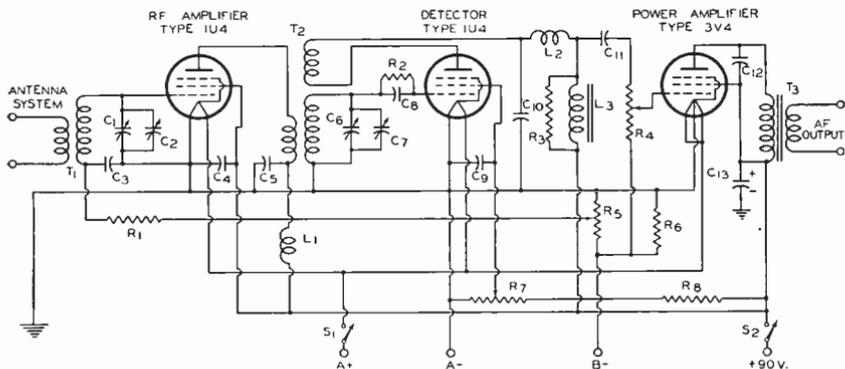
$C_1, C_2$  = Midget tuning capacitors, 140  $\mu\mu\text{f}$
