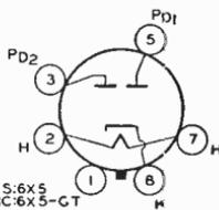
used principally for renewal purposes. Both types require octal socket. Type 6X5 should be mounted in vertical position, but horizontal operation is permissible if pins 3 and 5 are in horizontal plane. Type 6X5-GT may be operated in any position. For maximum ratings, typical operation data, and curves, refer to type 6X4.
