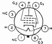
octal socket and may be mounted in any position. Heater volts (ac/dc), 25; amperes, 0.3. Except for heater rating, this type is identical with glass octal type 6BQ6-GT.
