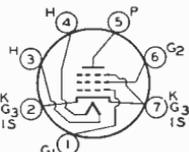
contact socket and may be mounted in any position. The two cathode leads facilitate isolation of the input and output circuits thus helping to minimize degeneration. For heater and cathode considerations, refer to type 6AV6.
