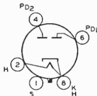
volts (rms), 700; total effective plate-supply impedance per plate, 50 ohms; dc output ma., 125. Typical operation with choke-input filter: ac plate-to-plate supply volts, 1000; minimum filter-input choke, 5 henries; dc output ma., 125.
