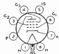
ma., 1.7; plate resistance, 0.75 megohm; transconductance, 1750  $\mu$ mhos; transconductance at bias of -40 volts, 10  $\mu$ mhos. The application of this type is similar to that of metal types 6SK7 and 6SS7.
