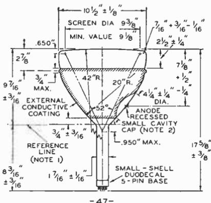
NOTE 1: Reference line is determined by position where gauge 1.500" + .003" - .000" I.D. and 2" long will rest on bulb cone.
