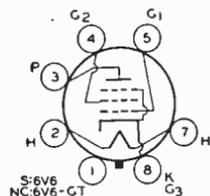
lines 6 and 22, respectively, **OUTLINES SECTION**. Tubes require octal socket and may be mounted in any position. The 6V6 and 6V6-GT are equivalent in performance to type 6AQ5. Refer to type 6AQ5 for heater and cathode considerations, application information, and characteristic curves.
