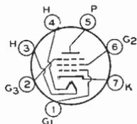
Miniature type used in compact equipment as a power amplifier. Outline 12, OUTLINES SECTION. Tube requires miniature seven-contact socket and may be mounted in any position. For heater and cathode considerations, refer to type 6AV6.
