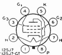
Heater volts (ac/dc), 12.6; amperes, 0.15. Except for heater rating, type 12SJ7 is identical with metal type 6SJ7, and type 12SJ7-GT is identical with glass-octal type 6SJ7-GT.
