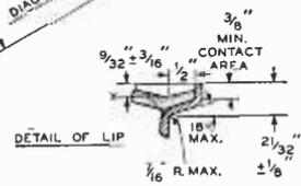
NOTE 1: With tube neck inserted through flared end of reference-line gauge (above) and with tube seated in gauge, the reference line is determined by the intersection of the plane CC' of the gauge with the glass funnel.
