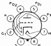
unit as class A<sub>1</sub> amplifier: plate volts, 250 *max*; plate dissipation, 2.5 *max* watts. For diode operation curves, refer to type 6SQ7.
