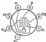
TION. Tube requires miniature seven-contact socket and may be mounted in any position. For heater and cathode considerations, refer to type 6AQ5.
