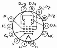
4000 *max*; anode-No.1 volts, 1500 *max*), this type is identical with type 7JP4. The 7JP4 may be used to replace the 7GP4 provided no connections are made to pins 4 and 12. The 7GP4 is a DISCONTINUED type listed for reference only.
