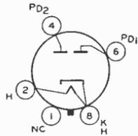
position. The heater is designed to operate from the ac line through a step-down transformer. The voltage at the heater terminals should be 5.0 volts under operating conditions at an average line voltage of 117 volts. It is especially important that this tube, like other power-handling tubes, should be adequately ventilated.
