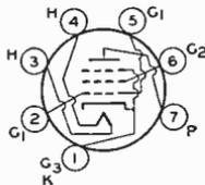
for terminal connections and slightly higher ratings, type 50C5 is equivalent in performance to miniature type 50B5 and, within its maximum ratings, to glass-octal type 50L6-GT. The basing arrangement of the 50C5 simplifies the problem of meeting Underwriters' Laboratories requirements in the design of ac/dc receivers.
