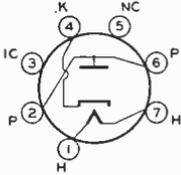
Miniature type used in power supply of small, portable, ac/dc/battery receivers where small size and low heat dissipation are important. Outline 12, OUTLINES SECTION. Tube requires miniature seven-contact socket and may be mounted in any position. This type is used principally for renewal purposes.
