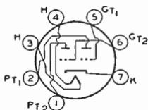
Miniature type used for converter service in ac/dc AM and FM receivers and as oscillator, amplifier, or mixer in television receivers of the "transformerless" type. Outline 12, OUTLINES
