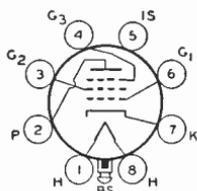
No.3 and internal shield connected to cathode at socket; plate resistance (approx.), 0.75 megohm; transconductance, 4200  $\mu$ mhos; grid-No.1 bias for plate current of 10  $\mu$ a, -10; cathode resistor, 250 ohms; plate ma., 6; grid-No.2 ma., 2. The application of this type is similar to that of miniature type 6BH6.
