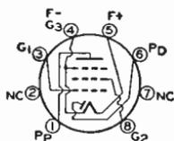
Subminiature type used as combined detector and audio amplifier in small, compact, battery-operated receivers for the standard AM broadcast band. The 1T6 and the other RCA
