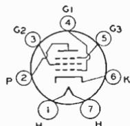
plate resistance, 2300 ohms; amplification factor, 6; transconductance, 2600; load resistance for maximum undistorted power output, 5000 ohms; undistorted output watts, 1.25. For typical operation as class A<sub>1</sub> amplifier (pentode connection; grid No.3 tied to cathode at socket), refer to type 6F6 with plate voltage of 250 volts. This type is used principally for renewal purposes.
