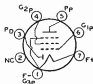
Miniature type used in light-weight, compact, portable, battery-operated receivers as combined detector and af voltage amplifier. Outline 12, OUTLINES SECTION. Filament volts (dc), 1.4; amperes, 0.05. Tube requires miniature seven-contact socket and may be mounted in any position. For electrical characteristics, curves, and application, refer to type 1U5.
