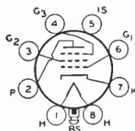
connected to cathode at socket; plate resistance (approx.), 1 megohm; transconductance, 3300  $\mu$ mhos; grid-No.1 bias for transconductance of 35  $\mu$ mhos, -20 volts; plate ma., 6.8; grid-No.2 ma., 1.9. The application of this type is similar to that of miniature type 6BJ6.
