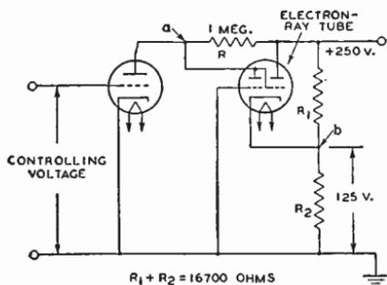
The choice between electron-ray tubes depends on the avc characteristic of the receiver. The 6E5 contains a sharp-cutoff triode which closes the shadow angle on a comparatively low value of avc voltage. The 6AB5/6N5 and 6U5 each have a remote-cutoff triode which closes the shadow on a larger value of avc voltage than the 6E5. The 6AF6-G may be used in conjunction with dc amplifier tubes having either remote- or sharp-cutoff characteristics.
