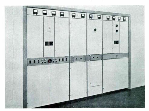
type 8FZ 511 broadcast equipment comprising from left to right: power supply, modulator, driver and final stage
