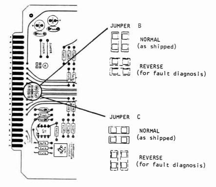
Fig. 2-2: Jumper Positions, OPTIMOD-FM Card #6
