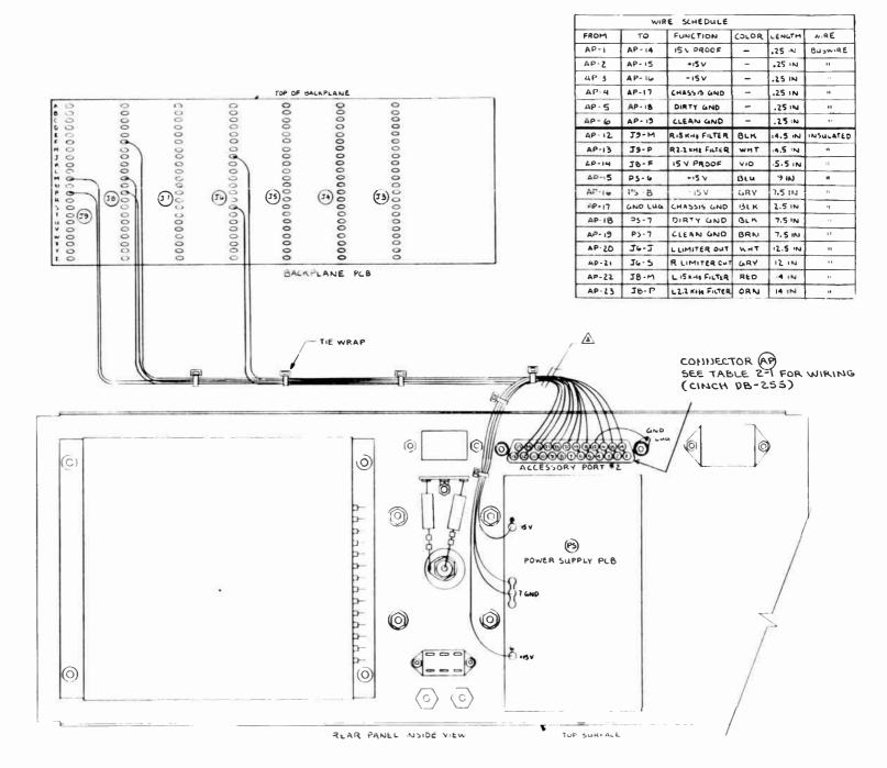
Fig. 2-4: Accessory Port #2 Installation
