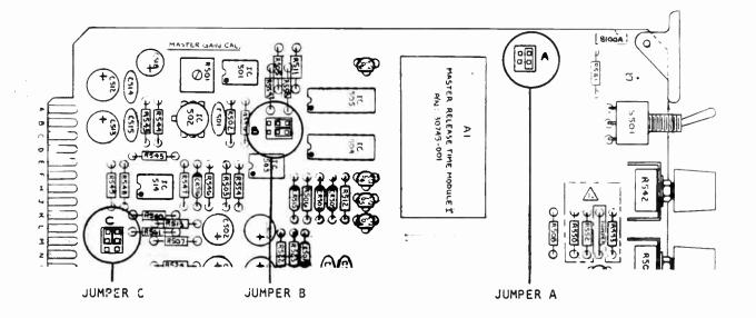
Fig. 2-6: Jumper Positions for Studio Chassis Alignment, Card #5 (Part number 30741-000-03 or above.)
