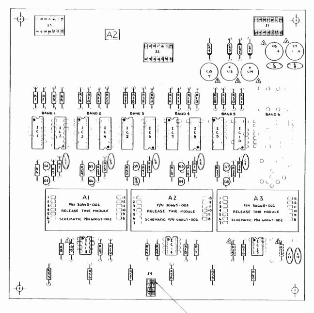
I. TICK MARKS INDICATE PIN ONE OF IC'S, MODULES; CATHODE OF DIDDES; POSITIVE SIDE OF CAPACITORS; EMITTER OF TRANSISTORS.
