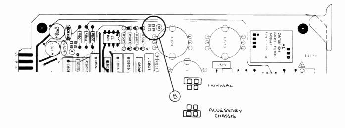
Fig. 2-3: Jumper Positions, OPTIMOD-FM Cards #8 and #9 (For Cards #8/#9, part numbers 30481-000-04 or above only – if your cards look different, see Appendix J of your OPTIMOD-FM Operating Manual for jumper locations.)
