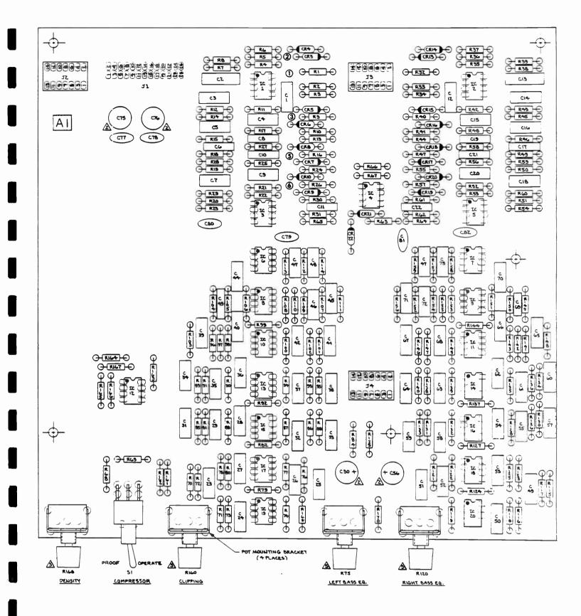
I. TICK MARKS INDICATE PIN ONE OF IC'S, MODULES; CATHODE OF DIDOUS; POSITIVE SIDE OF CAPACITORS; EMITTER OF TRANSISTORS.
