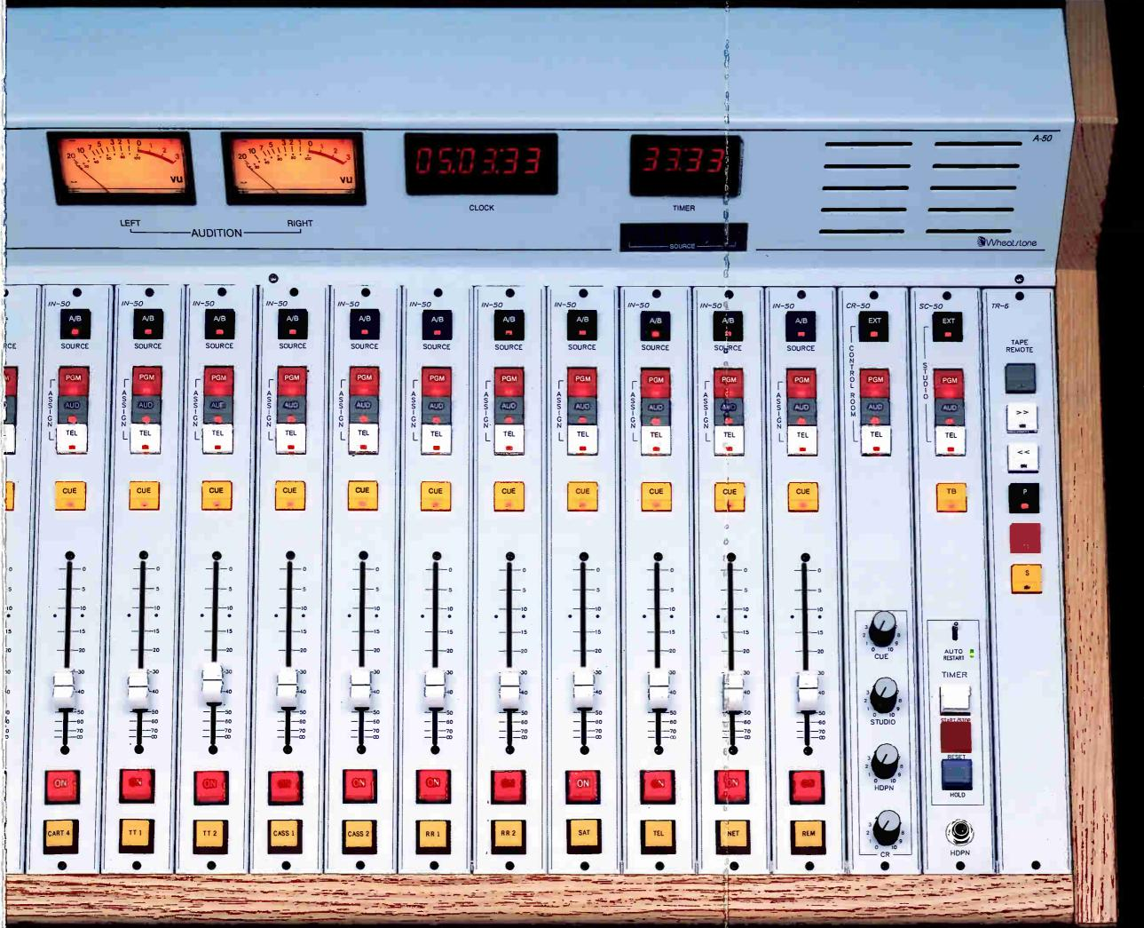
**CONTROL ROOM MUTE** - CR mic module is dipswitch selected to mute control room when CR mic is ON. This mute function prevents control room feedback when monitor speakers are utilized.
