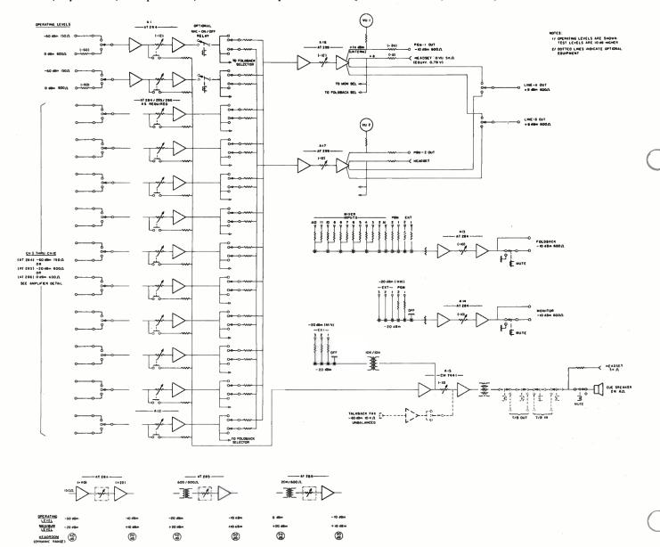
1 and 2 are normally wired for one low-level input (-60 dBm, 150 ohms) and one high-level input (0 dBm, 600 ohms); an optional microphone relay may be provided in each of these channels. By choice of amplifiers, nominal input levels of -60 dBm, -20 dBm, and 0 dBm may be accommodated in any mixer channel.
