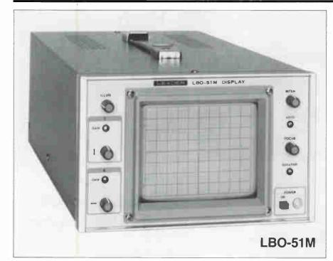
The LBO-51M is an X-Y CRT display designed primarily for use in OEM applications.
