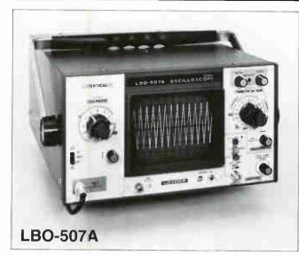
The single trace LBO-507A and the dual trace LBO-508A are both economical and versatile ... proven performers for a wide range of lab and field work. Both oscilloscopes offer 17.5-nsec rise time, 18 calibrated sweep speeds and a full range of triggering options. The add and subtract modes of the dual trace LBO-508A permit differential, phase-shift, and similar measurements. Both have a 5-inch CRT with 8 x 10-cm graticule.
