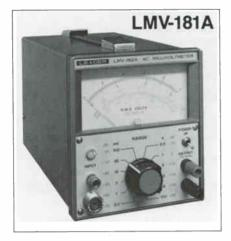
The LMV-181A and LMV-185A are general purpose average responding ac voltmeters with a measurement range-of 100 uV to 300 V. The LMV-182A is an average responding ac voltmeter with increased sensitivity featuring an effective measurement range of 30 uV to 100 V. Bandwidth is 5 Hz to 1 MHz permitting use in a broad range of applications including audio, IF and ultrasonic circuits and systems.
