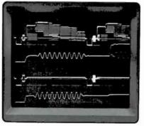
The alternate time-base mode permits viewing the main and delayed time bases for both channels simultaneously. The main time-base is shown with the delayed time-base portion intensified.
