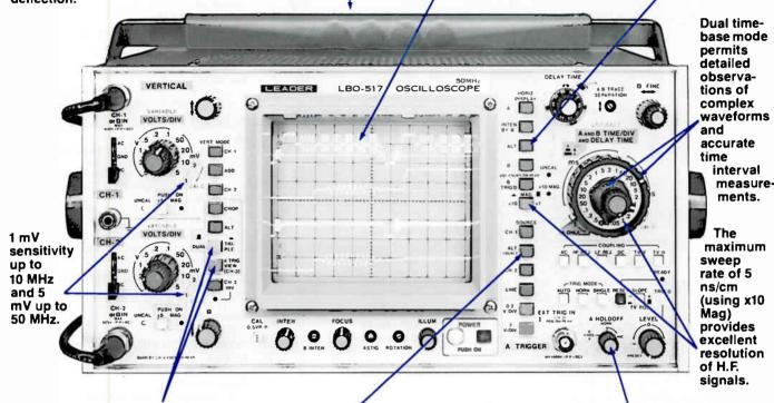
Third and fourth channel trigger view permits observing both the main and delayed time-base trigger wave forms. Channel 4 (input and position control on rear panel) may be used as an additional independent display channel when the delayed time-base is not triggered.
