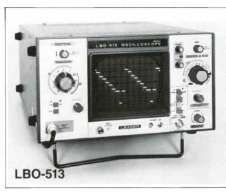
The single trace LBO-513 and the dual trace LBO-514 are compact 5-inch oscilloscopes that offer maximum performance at low cost. Equipped with both vertical and horizontal magnifiers, they have 1-mV sensitivity with X5 magnification and a maximum sweep speed of 0.1  $\mu s/cm$  (0.2 s/cm to 0.5 usec in 18 calibrated steps plus X5 magnification). Rise time of both oscilloscopes is 35 ns with normal and automatic, + or - triggering. The LBO-514 provides both chop and alternate dual trace displays
