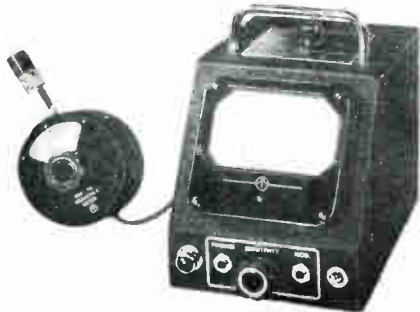
MODEL 59 MEGACYCLE METER 2.2 to 400 megacycles in seven coil ranges
