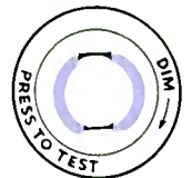
SHUTTERS CLOSED Minimum indirect "halo" light
