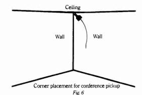
Install the capsule/holder in an upper corner of the room as in Fig. 6. This arrangement increases microphone output by 12 dB and gives surprisingly clear reproduction. Large rooms may require such a pickup in all four corners.
