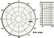
The GLM<sup>™</sup>-200 is a miniature electret-condenser hypercardioid microphone with excellent response and uniform off-axis rejection. Its sub-miniature size makes it almost invisible in actual use.
