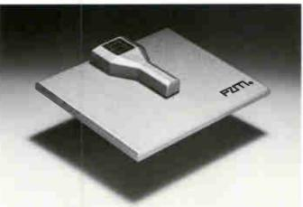
The 6 series PZM<sup>®</sup>s are designed for minimum visibility. A miniaturized cantilever and plate optimize the omnidirectionality (hemispherical pattern) of these units. Miniaturized electronics are housed in the XLR-type connector at the end of the cable. allowing direct interface to phantom powering.
