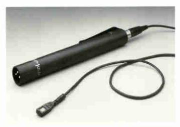
The GLM<sup>™</sup>-100/ENG is a miniature electret lavalier microphone specifically designed for ENG (electronic news gathering) uses. The frequency response of the ENG version is intentionally tailored to roll off the low frequency response to avoid rumble and much of the normal ambience found in ENG outdoor work.
