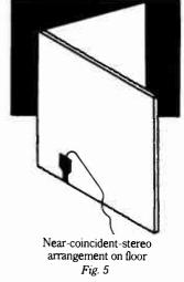
This assembly can be suspended, or can be placed on edge on the floor, with the PZMs at the junction of the floor and the vertical panels (as in Fig. 5).
