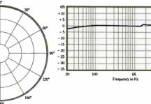
Horizontal Plane Polar Response source 30° above infinite boundary
