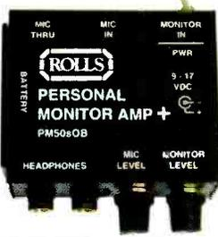
Rolls also offers the PM50s and PM50sOB (optional battery) Personal Monitor Amps. These units mix a 1/4" TRS stereo monitor signal with an XLR microphone signal. They make the perfect "more me" box - you mix your own voice/ instrument with the main mix.
