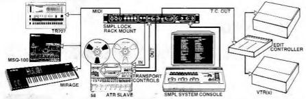
In the full Audin/Video production, SMPL Lock's Chase Mode allows Audio Transports to Chase and follow the action of two or more VTRs in a Video Editing Suite. All basic SMPL System functions as well as MIDI are retained
