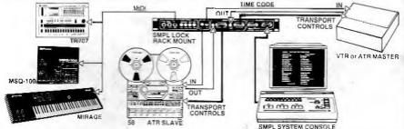
The addition of the Lock Extension allows for Sync Lock control of the two transports and full MIDI Locate and Lock. All basic SMPL System functions and features are retained. Ideal for the needs of the independent finale writer or studios sceking to gain tracks by locking audio transports.
