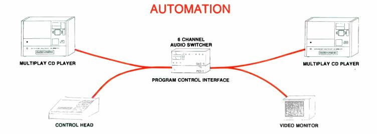
AUTO MODE OPERATION — In the AUTO mode the AMCDS — 1000A is controlled by an external programmer, the SMC-CDP (Live Assist/Music Retrieval). This programmer provides the required DISC and CUT data to the AMCDS — 1000A, which in turn, will send the following data back to the programmer:
