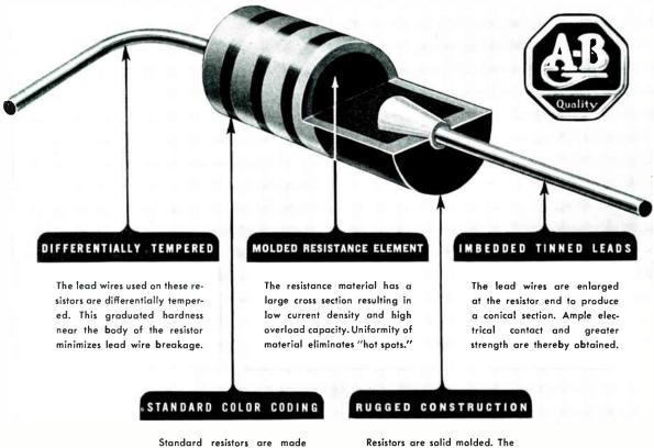
in all RETMA, JAN, and MIL specifications, resistance values, and color coding. Tolerances plus or minus 5%, 10% or 20%. Resistors are solid molded. The resistance material, insulation material and lead wires are molded together at one time into **a** solid integral structure.
