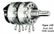
The rotating mechanism which is attached to the operating shaft consists of a metal actuator provided with insulation which supports the pressure spring. The latter maintains the movable composition contact brush in intimate contact with the resistance track and also provides electrical connection between the brush and the collector ring which is molded as an integral part of the element.
