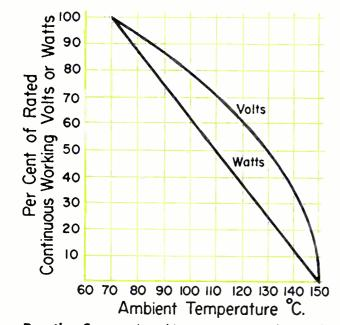
**Derating Curve** – At ambient temperatures above  $70^{\circ}$ C the change in resistance, after 1000 hours, will be less than 6% provided the working voltage is derated in accordance with the above curve.
