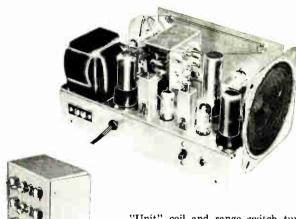
"Unit" coil and range switch turret assembly completely assembled and wired by the kit builder before installation in the chassis. Copper plated coil mounting with aluminum shield plate.
