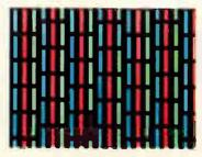
New slot-mask picture tube for greater light output and picture realism.
