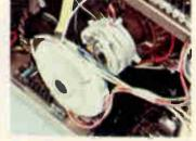
New static toroid yoke & factory-adjusted & sealed assembly end convergence or purity adjustment — forever.
