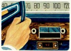
Digital Speedometer - Reads 0-99 miles per hour on amberorange digital readout
