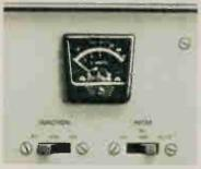
Versatile front panel meter shows signal strength on receive, ALC voltage on transmit, switches to read relative power output or final amplifier cathode current.
