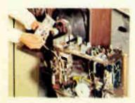
Modular circuit boards plug onto the slide out chassis for really easy servicing.
