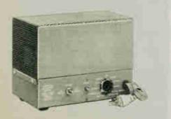
Provides the operating voltages needed for fixed station transceiver use — high voltage, two low voltages, fixed bias, 12.6 volt filament. The improved HP-23B now features a higher voltage rating on B + filter capacitors; improved filtering on bias voltage; fixed bias voltage, and heavier filament wires in the power cable. Now the popular Heathkit power supply is better than ever.
