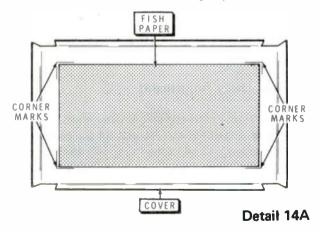
() Refer to Detail 14A and remove the white, protective covering from the fish paper. Lower the adhesive side of the paper carefully onto the inside of the cover. Use
