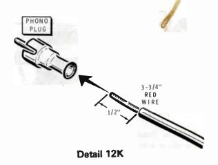
() Refer to Detail 12K and insert the 1/2" bare end of a red wire into a phono plug. Heat the tip of the phono plug with a soldering iron and solder the wire to the plug tip. Carefully shave off any solder on the outside of the plug tip with a knife. Cut off any excess lead protruding from the tip of the plug.
