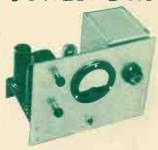
A variable power supply is a most convenient tool around any shop. This simple supply can be varied between 80 and 300 volts with only one 100,000 ohm potentiometer. The control tubes may be surplus 1619 tubes or 6L6 and the two control tubes will pass up to 100 MA. The photos show a sample built up by the Heath Company. The layout is not important and may suit the builders material.
