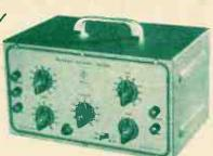
60 cycle transformer operated. Uses 5 tubes (1 6X5, 2 6SN7's, 2 6SI7's). Has individual gain controls, positioning control and coarse and fine sweeping rate controls. The cabinet and panel match all other Heathkits. Every part supplied including detailed instructions for assembly and use. Shipping Wt. 11 lbs.
