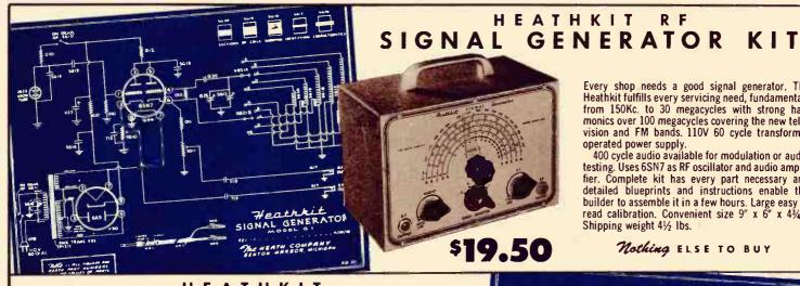
Every shop needs a good signal generator. The Heathkit fulfills every servicing need, fundamentals from 150Kc. to 30 megacycles with strong harmonics over 100 megacycles covering the new television and FM bands. 110V 60 cycle transformer operated power supply.
