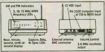
An RF receiver scans the 5, 10 and 15 MHz frequencies of WWV and locks onto the strongest signal. A mutable audio monitor permits listening to the audio broadcasts on these frequencies. An external antenna is recommended but may not be required in your area.
