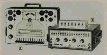
1 Low-Cost Heathkit Tube Checker. Essential for radio-TV servicing! Tests tubes on the basis of total emission, for shorts, leakage, open elements, and filament continuity. Has good/bad indicator to show relative quality, neon bulb indicator for filament continuity and leakage or shorts between elements.
