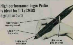
Detects and indicates high and low logic levels in TTL or CMOS circuitry. Detects logic signals to 100 mHz, polarity and presence of single pulses as short as 10 nSec. Memory indicator shows any transition in logic level. Includes power leads, mini-clips and ground clip. 34" H x 1" W x 91/4" L.
