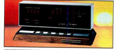
ID-1990 SPECIFICATIONS: Barometer Display: 4-digit readout. Separate indicators show whether the pressure is rising or falling, and whether the display is in mches of mercury, millibars or kiloPascals. Pressure Ranges: 28.00 to 32.00 inches Hg (mercury), 981 to 1050 millibars or 98.1 to 105 kiloPascals. Accuracy: 29.00 to 31.00 Hg  $\pm$  0.03 in. Hg at 15-35° C. Power: 120/240 VAC.
