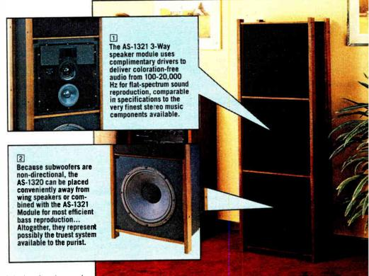
AS-1320 SPECIFICATIONS: Freq. Range (-10 dB anechoic): 15-750 Hz. Freq. Response (±3 dB): 22-500 Hz. Impedance: 8Ω. Minimum Amplifier Power: 30 W. Maximum Power: 250 W. Driver: High compliance, 15" long-throw design, Cabinet Type: Nine-cubic-foot vented box, tuned to 22 Hz using computer-aided modeling techniques. Cabinet Dimensions: 64½" H x 21½" W x 17" D.
